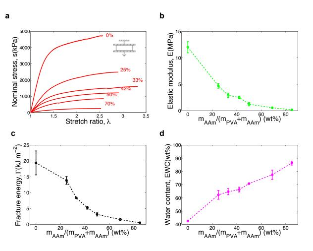
Figure 3. Composition greatly affects the properties of the hybrid gel. **a**, Stress-stretch curves of hybrid gels of various weight percentages of acrylamide to (acrylamide plus polyvinyl alcohol), as labeled. **b**, Elastic modulus, *E*, derived from the initial slope of the stress-stretch curves. **c**, Fracture energy,  $\Gamma$ , as a function of the acrylamide content. **d**, Water contents of the gels fully swollen in distilled water, *EWC*, plotted against the acrylamide content.
