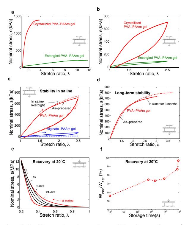
**Figure 2.** Crystallites as stable and recoverable cross-links. **a**, Stress-stretch curves of two types of gels. Each sample is stretched to rupture. The nominal stress is the applied force divided by the cross-sectional area of the undeform sample. The stretch ratio is the length of deformed sample divided by the initial length. **b**, Loading-unloading curves of both gels. Each sample is
