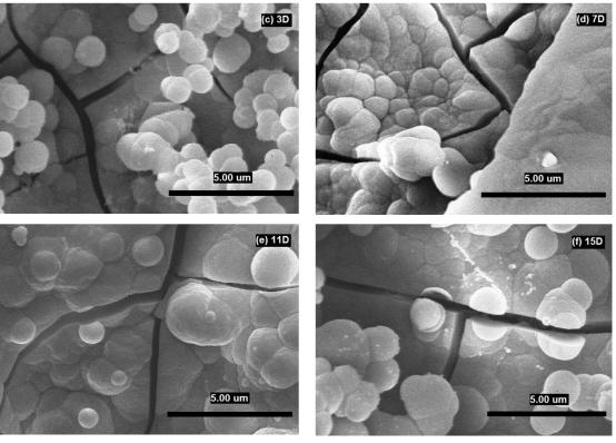
**Fig. 6.** SEM images of scaffolds (a) before (combette - the small tabular crystals, buchwaldite and structurally isomorphic phase CaO.SiO<sub>2</sub> - needle-like crystals) and after (b) 1, (c) 3, (d) 7, (e) 11 and (f) 15 days of interaction with I-solution. The fractures in the newly developed layers were caused by drying of samples.
