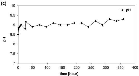
**Fig. 4**. Concentrations of (a) Si, (b) Ca<sup>2+</sup>, (PO<sub>4</sub>)<sup>3-</sup> ions and (c) values of pH in I-solution during interaction with scaffolds
