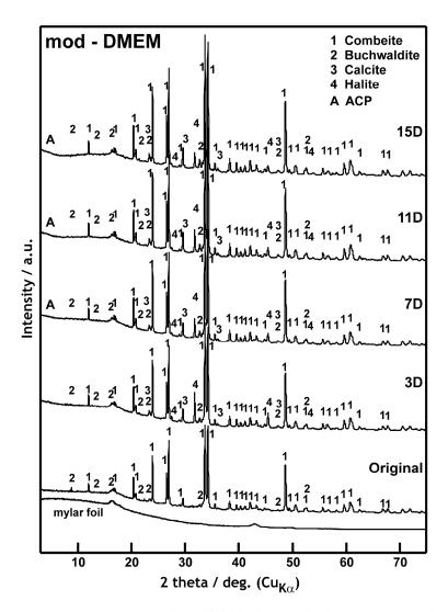
**Fig. 2.** XRD patterns of scaffold before and after 3, 7, 11 and 15 days of interaction with mod-DMEM
