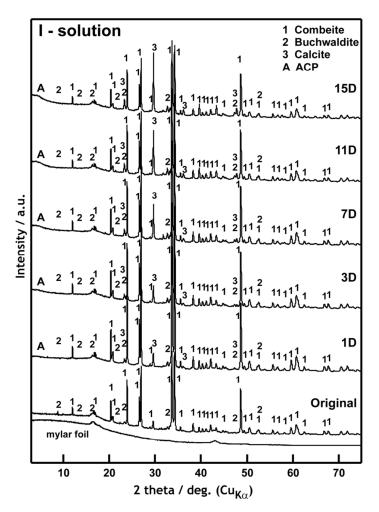
**Fig. 5.** XRD patterns of scaffolds before and after 1, 3, 7, 11 and 15 days of interaction with I-solution
