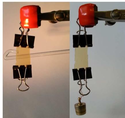
**Fig. 1** Appearance of the films based on semi-IPN architecture: photograph of the transparent semi-IPN2 with and without the load.
