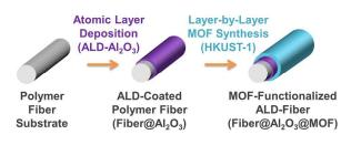
**Scheme 1.** Schematic of the synthesis route. Polymer fiber substrates were coated with 50 cycles of ALD-Al<sub>2</sub>O<sub>3</sub>, forming a core@shell structure of "Fiber@Al<sub>2</sub>O<sub>3</sub>". HKUST-1 MOF thin film was grown onto ALD-coated polymer fibers via layer-by-layer synthesis method.
