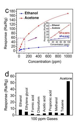
Fig. 5 (a) Sensor responses of CuO-ZnO/rGO towards acetone and ethanol; (b) The  $S_{acetone}/S_{ethanol}$  of CuO-ZnO/rGO vs. gas concentrations; (c) The sensitivity tendency of CuO-ZnO/rGO vs. different gas concentrations, the inset shows corresponding calibration curves (10 to 100 ppm); (d) The response of CuO-ZnO/rGO sensor to 100 ppm of various VOCs gases.
