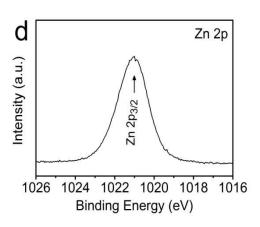
**Fig. 2** XPS survey of (a) whole scan spectrum; (b) deconvoluted C 1s of CuO-ZnO/rGO, the insert of (b) is deconvoluted C 1s of GO; (c) Cu 2p of CuO-ZnO/rGO; (d) Zn 2p of CuO-ZnO/rGO.
