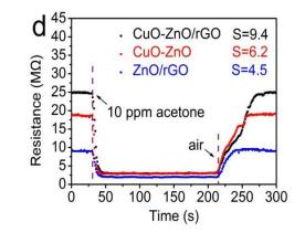
**Fig. 4** (a) The response of CuO-ZnO/rGO sensor to 10 ppm of acetone vs. operating temperatures; (b) The response transients of CuO-ZnO/rGO sensor to 10 ppm of acetone, the inset of (b) depicts the details of once adsorption and desorption; (c) Current–voltage (I–V) characteristics of CuO-ZnO/rGO, CuO-ZnO and ZnO/rGO sensors at room temperature; (d) The resistance curves of CuO-ZnO/rGO, ZnO–CuO and ZnO/rGO sensors to 10 ppm of acetone.
