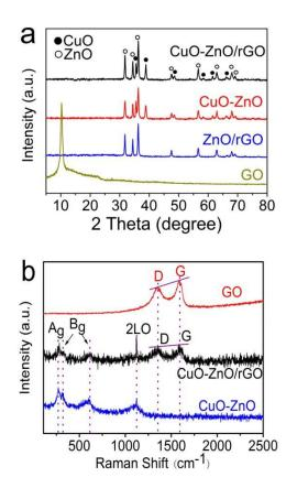
**Fig. 1.** (a) XRD patterns of CuO-ZnO/rGO, CuO-ZnO, ZnO/rGO and GO; (b) Raman spectra of GO, CuO-ZnO/rGO and CuO-ZnO.
