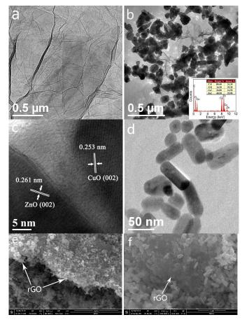
**Fig. 3** TEM or HRTEM images of (a) GO, (b, c) CuO-ZnO/rGO and (d) CuO-ZnO, the insert of (b) is EDS spectrum of CuO-ZnO/rGO; (e, f) FESEM of CuO-ZnO/rGO.
