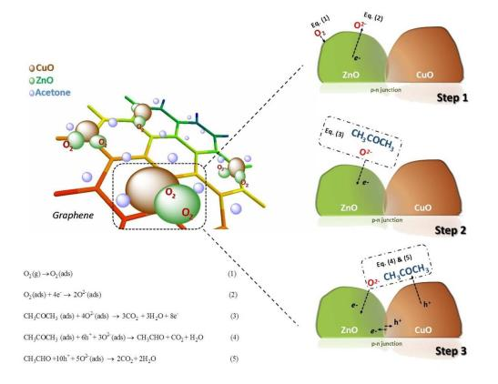
Fig. 6 Schematic diagram of the proposed mechanism of CuO-ZnO/rGO.
