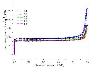
Fig. 9  $\mathrm{N}_2$  adsorption/desorption isotherms of as-synthesized nano SAPO crystals.
