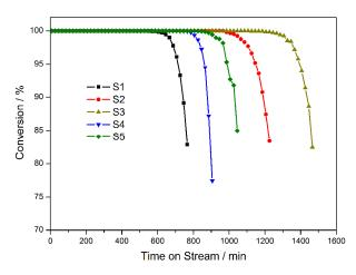
s **Fig. 11** Methanol conversion variation with time-on-stream over nano SAPO catalysts with different silicon contents. Experimental conditions: WHSV =  $2 h^{-1}$ , T = 400 °C, catalyst weight = 300mg.
