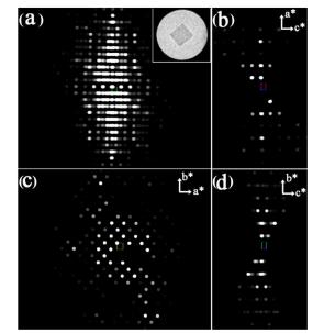
**Fig. 4** Reconstructed 3D reciprocal space of phase **2**. (a) The whole set of 3D EDT data (inset: the image of the crystal), (b) h0l plane, (c) hk0 plane, 60 and (d) 0kl plane cut from 3D reciprocal space.
