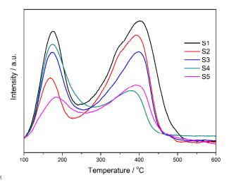
Fig. 8 NH<sub>3</sub>-TPD profiles of as-synthesized nano SAPO crystals.
