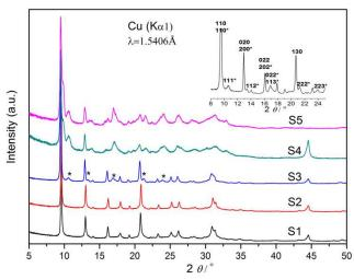
Fig. 1 Powder XRD patterns of as-synthesized nano SAPO crystals. S1: CHA-type; S2: CHA-type; S3: CHA-type/AEI-type; S4: CHAtype/AEI-type; S5: AEI-type. Asterisks denote reflections only from 5 AEI-type. Range of 8°-25° of S3 is indexed (inset on the right top corner).
