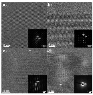
**Fig. 6** HRTEM images and corresponding SAED patterns along (a) [001] (CHA-type /AEI-type), (b) [100] (AEI-type), (c) [010] (CHA-type) and (d) [110] (AEI-type & CHA-type) directions. The white arrows in c and d s show the existence of defects.
