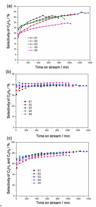
Fig. 12 Products distributions over nano SAPO catalysts with different silicon contents. Experimental conditions: WHSV =  $2 h^{-1}$ , T = 400 °C, catalyst weight = 300 mg. (a) selectivity of C<sub>2</sub>H<sub>4</sub>, (b) selectivity of C<sub>3</sub>H<sub>6</sub>, and (c) selectivity of C<sub>2</sub>H<sub>4</sub> and C<sub>3</sub>H<sub>6</sub>.
