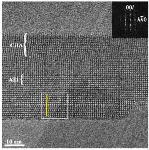
**Fig.** 7 TEM image of the S3 crystal with intergrowth of two types of framework. The inset on the top right corner is Fourier transformation of the area marked by the white square.
