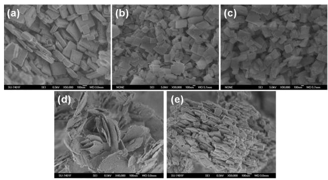
Fig. 2 SEM images of as-synthesized nano SAPO crystals. (a) S1; (b) S2; (c) S3; (d) S4; (e) S5. Scale bar in (a)-(e): 100 nm
