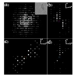
Fig. 3 Reconstructed 3D reciprocal space of phase 1. (a) The whole set of <sup>55</sup> the 3D EDT data (inset: the image of the crystal), (b) *h0l* plane, (c) *hk0* plane, and (d) 0*kl* plane cut from 3D reciprocal space.
