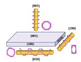
Scheme 1 Diffusion of methanol and generated products through 3D 8ring channels along the [100], [010], and [001] direction of nano sheet-<sup>75</sup> like SAPO-34 crystal.
