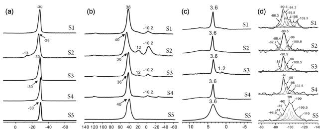
**Figure 10.** (a) <sup>31</sup>P, (b) <sup>27</sup>Al, (c) <sup>1</sup>H, and (d) <sup>29</sup>Si, MAS NMR (solid line) spectra of as-synthesized nano SAPO crystals.
