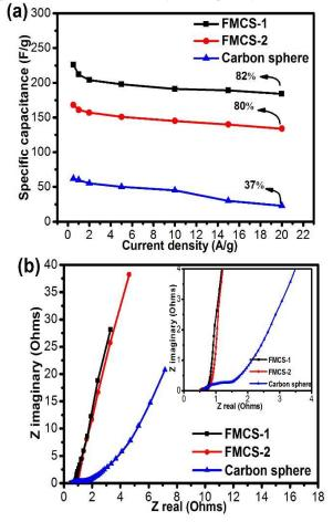
Fig. 9 (a) Corresponding specific capacitances of FMCS and carbon sphere at different current densities; (b) Nyquist plots of electrodes based on FMCS and carbon sphere.
