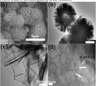
Fig. 5 (a) SEM, (b,c) TEM and (d) HRTEM images of FMCS-1. The presence of mesopores is indicated by the white arrows.
