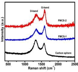
Fig. 7 Raman spectra of 3D FMCS and carbon sphere.
