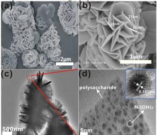
Fig. 2 (a,b) SEM, (c)TEM and (d)HRTEM images of the product of 15 hydrothermal reaction.
