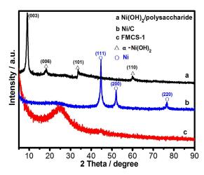
Fig. 3 XRD patterns of (a) Ni(OH)<sub>2</sub>/polysaccharide precursor, (b) Ni/C composite and (c) FMCS-1.
