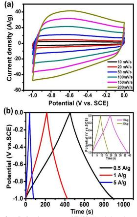
Fig. 8 (a) Cyclic voltammograms of FMCS-1 based electrode at various scan rates. (b) Charge/discharge curves of FMCS-1 based electrode at various current densities.
