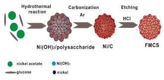
Fig. 1 Schematic illustration of the preparation of 3D FMCS.
