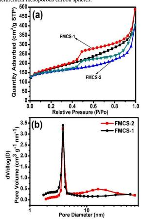
55 Fig. 6 (a) Nitrogen adsorption-desorption isotherms and (b) pore size distribution curve of the FMCS.
