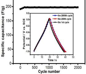
Fig. 10 The cycling performance of FMCS-1 electrodes at the current density of 10 A/g (inset: the charge/discharge curves for the 1st, 200th and 2000th cycles).
