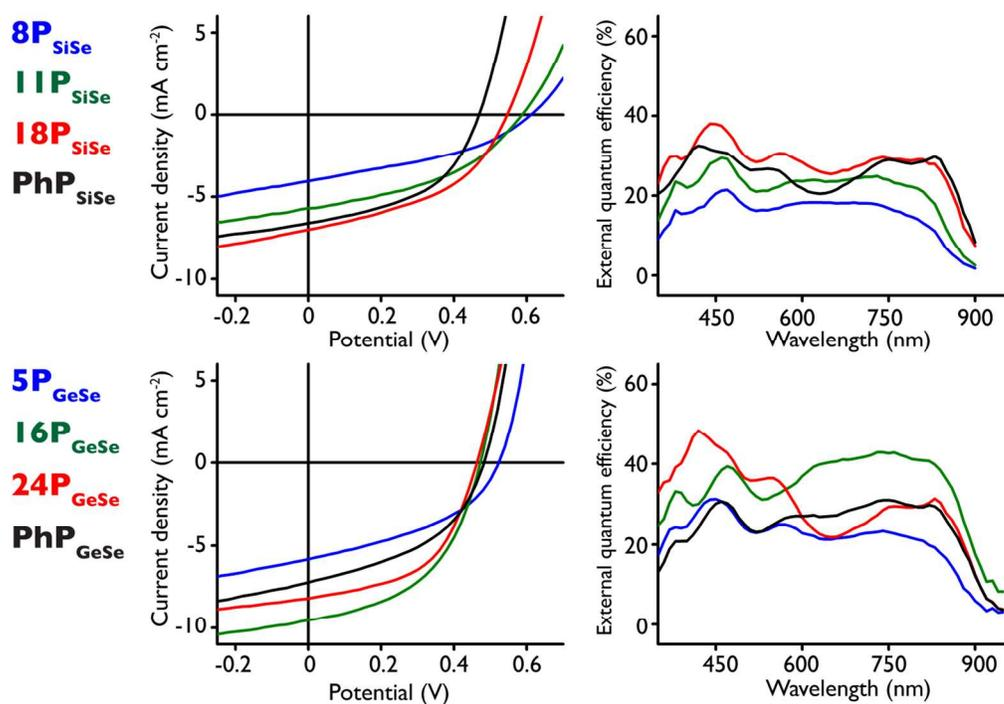
**Fig. 4** (top left)  $P_{SiSe}$  series  $J-V$  curves; (top right) corresponding  $P_{SiSe}$  series EQE curves; (bottom left)  $P_{GeSe}$   $J-V$  curves; (bottom right) corresponding  $P_{GeSe}$  EQE curves.
