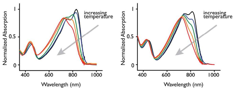
**Fig. 2** (left)  $^{33}\text{P}_{\text{SiSe}}$  and (right)  $^{24}\text{P}_{\text{GeSe}}$  absorption spectra in chlorobenzene ( $\sim 10^{-6}$  M) collected at 20 °C (black), 40 °C (blue), 60 °C (green), 80 °C (orange) and 100 °C (red).
