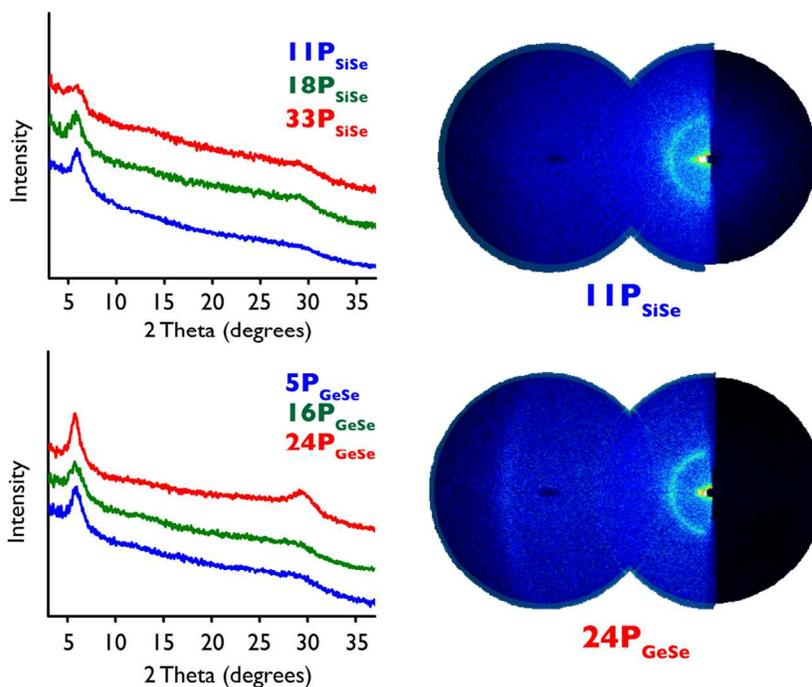
**Fig. 3** (top left) Radially averaged  $\mathbf{P}_{\text{SiSe}}$  traces from film 2-D WAXS plots; (bottom left) radially averaged  $\mathbf{P}_{\text{GeSe}}$  traces from film 2-D WAXS plots; (top right)  $\mathbf{11P}_{\text{SiSe}}$  2-D WAXS plot as a representative example; (bottom right)  $\mathbf{24P}_{\text{GeSe}}$  2-D WAXS plot as a representative example; all films drop cast onto silicon substrates from chlorobenzene solution and annealed for 30 min at 130 °C.
