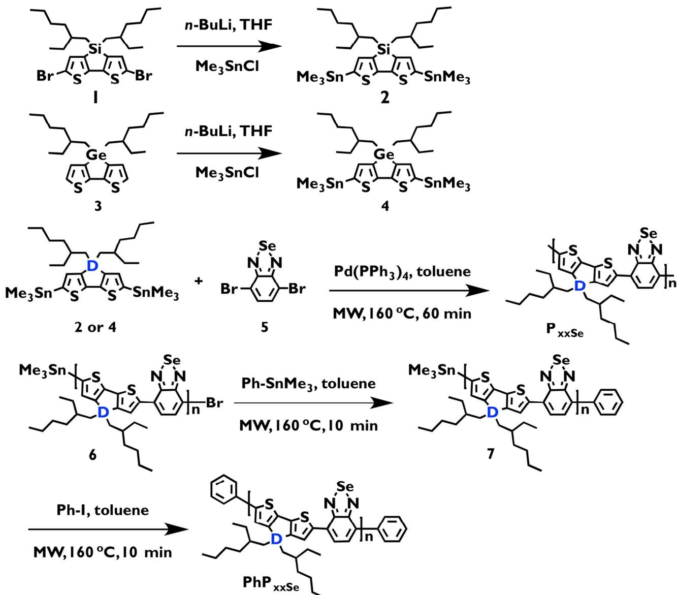
**Scheme 1** Synthesis of heavy atom monomers and corresponding 2,1,3-benzoselenadiazole-containing polymers P<sub>SiSe</sub> (D = Si), P<sub>GeSe</sub> (D = Ge); MW = microwave.
