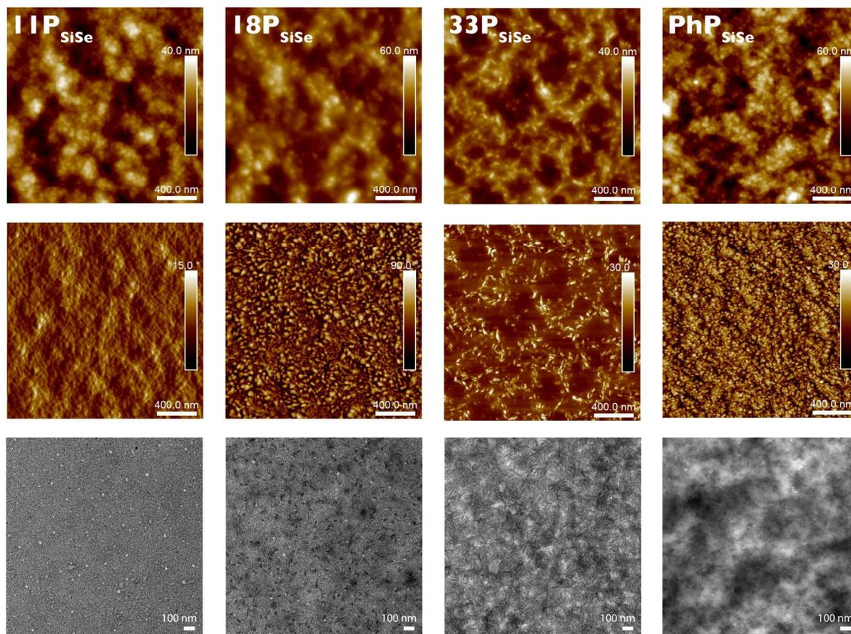
**Fig. 5** (top row)  $P_{SiSe}/PC_{71}BM$  blend film AFM height images; (middle row) AFM phase images; (bottom row) TEM images at 10 000x magnification; columns are labeled with the specific polymer blended with  $PC_{71}BM$  in the top panel; AFM data were collected directly on the device film between surface electrodes; TEM films were cast from 5 mg/mL polymer/ $PC_{71}BM$  solutions in chlorobenzene onto PSS coated glass slides, delaminated in water and collected onto a TEM grid.
