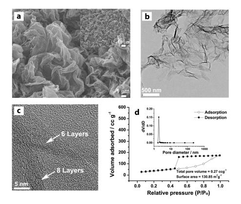
**Fig. 2.** (a) SEM and (b) TEM images of NSG nanosheets showing highly folded morphology due to the structural defects induced by the co-doping of heteroatoms. The inset in (a) shows a low-magnification SEM image of NSG nanosheets. (c) HR-TEM image of an NSG nanosheet showing the folded regions. (d) Nitrogen adsorption/desorption isotherms of the NSG sample. The inset shows that the pore size of NSG sample was ~2 nm, implying that the NSG sample has a mesoporous structure.
