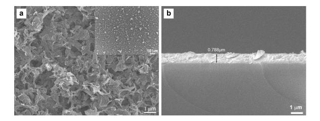
**Fig. 5**. (a) A representative SEM image of NSG counter electrode electrosprayed on a FTO glass and the inset shows the low-magnification SEM image. (b) Cross-sectional SEM image of NSG counter electrode.
