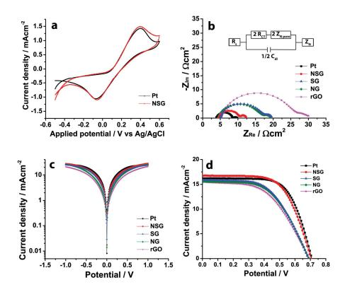
**Fig. 6**. (a) CV curves of NSG and Pt electrodes obtained at a scan rate of 50 mV s<sup>-1</sup> using Pt wire and Ag/Ag<sup>+</sup> as counter and reference electrodes, respectively. (b) Nyquist plots of different counter electrodes using symmetric cells. (c) Tafel polarization curves of different counter electrodes using symmetric cells. (d) Photocurrent-voltage curves of DSSCs with different counter electrodes under one-sun illumination.
