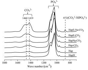
Fig.6 IR spectra of HAPs in the 700-1800 cm<sup>-1</sup> region.
