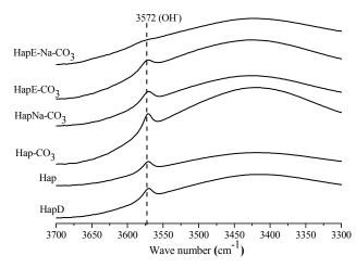
Fig.7 IR spectra of HAPs of the carbonate apatites in the 3300-3700 cm<sup>-1</sup> region.
