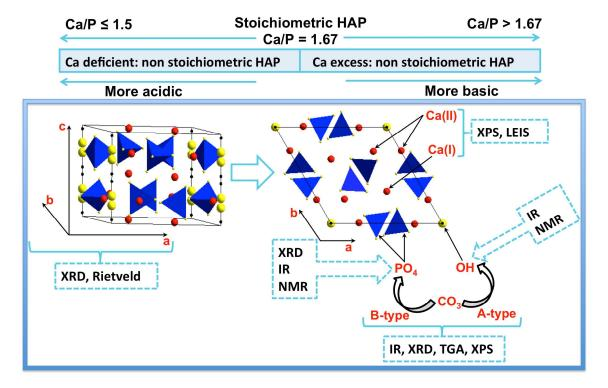
HAP solids were prepared by modifying their Ca/P ratio and by introducing Na<sup>+</sup> cations before being extensively characterized by XRD, XPS, LEIS, NMR, IR, TGA... Their acid base properties were then measured and discussed in relation with the characterization results.
