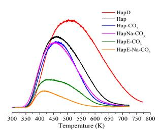
Fig.11 NH<sub>3</sub>-TPD curves of the apatite solids.
