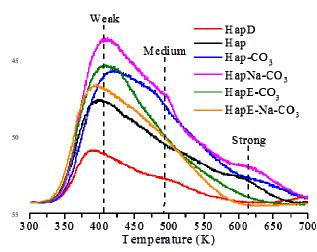
Fig.14 CO<sub>2</sub>-TPD profiles of the apatite solids.
