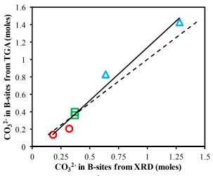
**Fig.5** Number of moles of CO<sub>3</sub><sup>2-</sup> in B-sites obtained from TGA as a function of the same parameter obtained from XRD (circles representing HapD and Hap, squares for carbonated apatites, namely Hap-CO<sub>3</sub> and HapNa-CO<sub>3</sub>, and triangles for carbonate-rich apatites, namely HapE-CO<sub>3</sub> and HapE-Na-CO<sub>3</sub>). The dashed line represents the theoretical perfect correlation (1 to 1 ratio).
