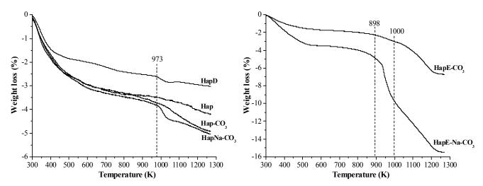
Fig.4 TGA curves showing the weight loss of the samples calcined at 673 K. The derived curves of  $CO_2$  loss obtained by using mass spectrometer with m/z = 44 are shown in Figure S5†.
