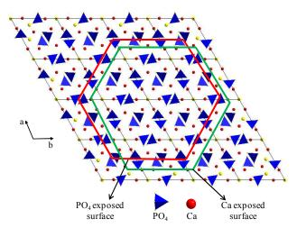
Fig.10 Schematic representation of the hydroxyapatite lattice: The green line shows the crystallite surface cleavage through Ca atoms, which is 10 actually occurring according to our study, and the red line shows the theoretical crystallite cleavage through P atoms that is another possibility, but not predominant in our solids.
