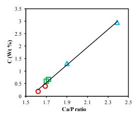
Fig. 1 Carbon content as a function of the bulk Ca/P ratio of the solids (circles representing HapD and Hap, squares for carbonated apatites, namely Hap-CO<sub>3</sub> and HapNa-CO<sub>3</sub>, and triangles for carbonate-rich apatites, namely HapE-CO<sub>3</sub> and HapE-Na-CO<sub>3</sub>).
