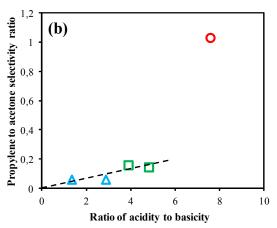
Fig.16 (a) Ratio of propylene to acetone selectivity as a function of the ratio between the number of acid sites to the number of basic sites and (b) Same figure focused on a narrower range of acidity/basicity ratio (red circles representing HapD and Hap, green squares for carbonated apatites, namely HapCO<sub>3</sub> and HapNa-CO<sub>3</sub>, and blue triangles for carbonate-rich apatites, namely HapE-CO<sub>3</sub> and HapE-Na-CO<sub>3</sub>).
