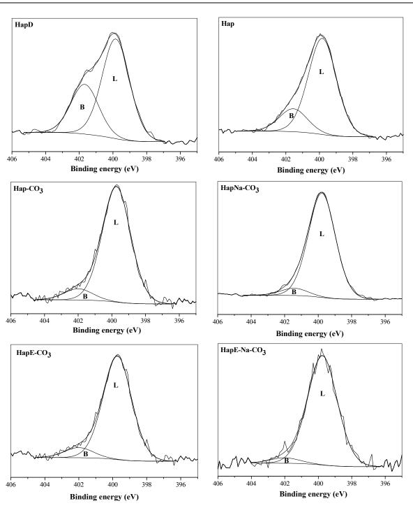
Fig.12 Decomposition of the N 1s photopeak after PEA adsorption on the apatite solids surface.
