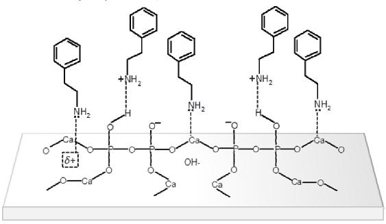
**Fig.13** Model of PEA adsorption over Lewis and Brønsted acid sites on the surface of apatites.  $[(\delta +)] = OH$  vacancies].
