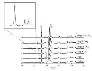
Fig.2 XRD patterns of the calcined solids.
