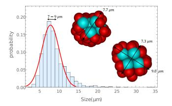
Fig. 7 Distribution of tube diameters obtained from optical microscopy, with a Gaussian fit (in red). The diameter is well-defined around 7 to 9  $\mu$ m. The insets show a cross-sections of the straight and spiral tube structures found in simulations, the diameters of which correspond to the peak in the distribution.
