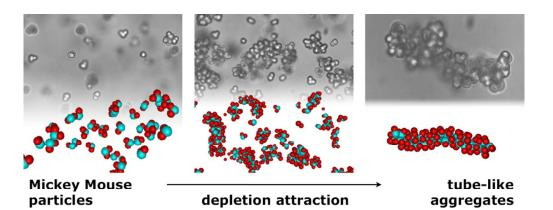
Triangular colloids with one sticky and two non-sticky lobes self-assemble into tube-like structures due to their geometry and anisotropic interactions.
