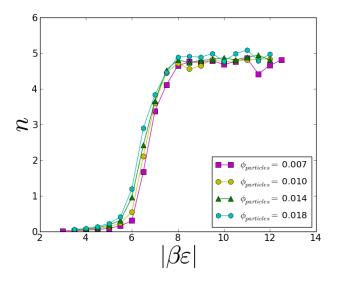
**Fig. 8** Average number of contacts per particle  $\langle n \rangle$  as function of the well depth of the attractive pair interaction, for different volume fractions  $\phi_{\text{particles}}$ . The figure shows a sharp transition from hardly any clusters at low interaction strength to a constant number of contacts (~5) for stronger interactions, irrespective of  $\phi_{\text{particles}}$ .
