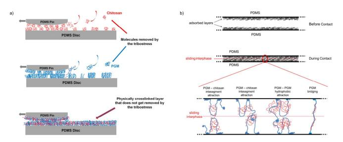
Fig. 6 a) Illustration of the tribostress-induced removal of the adsorbed layers from the PDMS surface and their resistance to it in the presence of chitosan, b) illustration of the chain interpenetration interactions between two PGM / chitosan layers.
