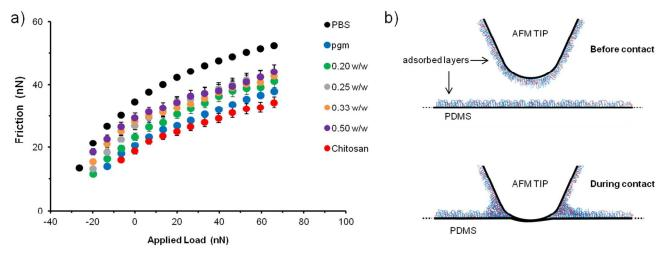
Fig. 7 a) Friction force microscopy data of 0.1 mg mL<sup>-1</sup> PGM, chitosan and their mixtures obtained from the contact between OTS silanized probes and PDMS slabs in the buffer solution (mixtures denoted according to the [chitosan] / [biopolymer] weight ratio, where [biopolymer] = 0.1 mg mL<sup>-1</sup>.), b) illustration of the plowing of the probe through the crosslinked network during FFM measurements.
