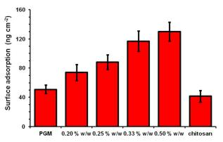
Fig. 4 Surface adsorbed masses on PDMS spin-coated waveguides of 0.1 45 mg mL<sup>-1</sup> PGM, chitosan, and their mixtures as characterized by optical waveguide lightmode spectroscopy (OWLS). Adsorption was allowed to occur for 30 minutes. Mixtures denoted according to the [chitosan]/[biopolymer] weight ratio, where [biopolymer] =  $0.1 \text{ mg mL}^{-1}$ .
