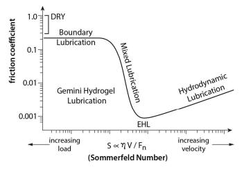
Fig. 1 (a) Schematic of a lubricated sliding interface with pertinent variables shown. (b) Classical lubrication regimes between two sliding surfaces. (c) Classical Stribeck curve with the Gemini hydrogel lubrication regime identified.
