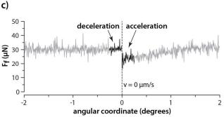
Fig. 2 (a) Schematic of a stationary hydrogel probe sliding against a rotating hydrogel disk in a Gemini hydrogel configuration. (b) Left: Normal  $(F_n)$  and friction  $(F_f)$  forces measured by capacitance sensors in the normal and the tangential direction, respectively, for a representative cycle (1 rotation). Right: The friction (tangential) force is two orders of magnitude lower than the corresponding normal force. (c) Friction forces for a representative cycle showing no static friction.
