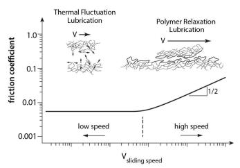
Fig. 5 Gemini hydrogel lubrication model. For low speeds, thermal fluctuation lubrication dominates and the coefficient of friction remains low. For high speeds, polymer relaxation and adhesion are the dominating mechanisms and a corresponding increase of friction coefficient to the ½ power arises.
