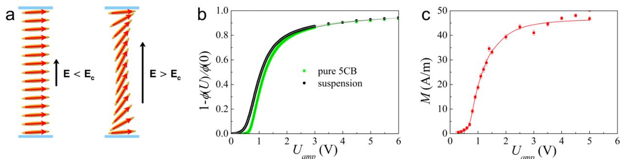
**Fig. 2** Electro-optic and converse magnetoelectric effects. a) A schematic of the director orientation  $\mathbf{n}$  (orange ellipsoids) and the magnetization  $\mathbf{M}$  (red arrows) below and above the critical electric field. b) Normalized phase difference vs applied voltage showing electro-optic response. c) Magnetization vs applied voltage showing converse magnetoelectric effect. The error bars indicate SEM. Lines are the fits (see text).
