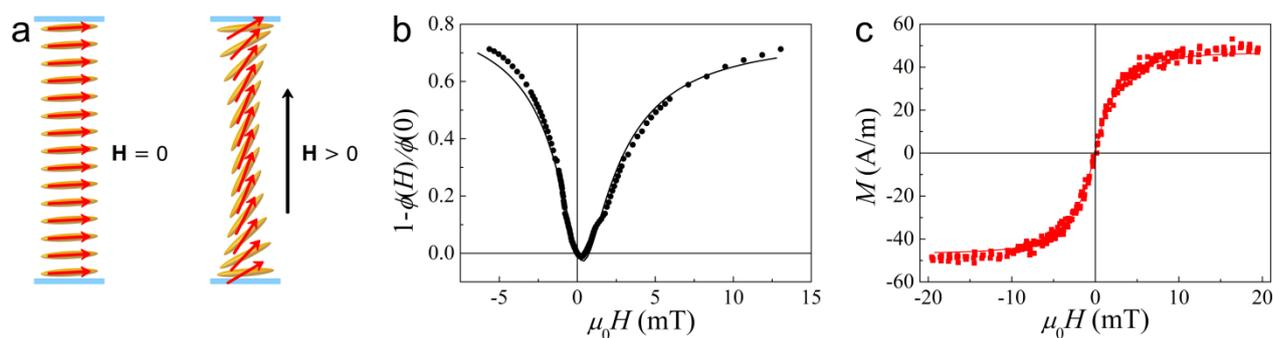
**Fig. 3** Magneto-optic effect in transverse field. a) A schematic of the director orientation  $\mathbf{n}$  (orange ellipsoids) and the magnetization  $\mathbf{M}$  (red arrows) with and without magnetic field. b) Normalized phase difference vs external magnetic field showing magneto-optic response. Pure 5CB remains undisturbed at these fields. c) Magnetization curve. Induced magnetization of pure 5CB is less than 0.1 A/m at these fields. Lines are the fits (see text).
