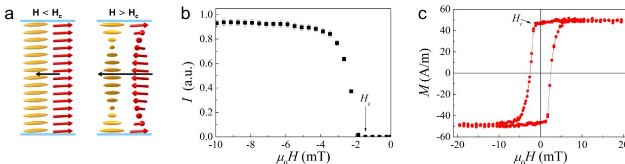
**Fig. 4** Magneto-optic effect in parallel field. a) A schematic of the director orientation  $\mathbf{n}$  (orange ellipsoids) and the magnetization  $\mathbf{M}$  (red arrows) below and above the critical magnetic field. b) Transmitted light intensity through the sample between crossed polarizers as measured by polarizing microscopy. Error bars indicate SEM. c) Magnetization curve.
