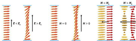
Schematics of converse magnetoelectric, transverse and parallel magneto-optic effects in a ferromagnetic liquid crystal.
