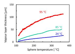
Vapour layer thickness vs sphere temperature for 20 mm superhydrophobic steel sphere cooling in 24 °C water (blue line), 85 °C (green line) and 95 °C water (red line), calculated using Fig. 2b data and eq. 4.
