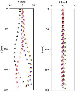
**Figure 7.** Examples of the trajectories of 40 mm steel falling spheres in 95 °C water: (a)  $T_s = 95$  °C hydrophilic spheres with no vapour layer, (b)  $T_s = 200$  °C superhydrophobic spheres in the Leidenfrost regime in the presence of a vapour layer. The horizontal and vertical (X, Z) trajectory coordinates are obtained from high speed video recording of five independent runs with each trajectory represented by a different symbol.
