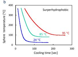
**Figure 2.** Sphere temperature *vs* cooling time for statically held 20 mm steel sphere cooling in 24 °C water (blue line), 85 °C (green line) or 95 °C water (red line): (a) hydrophilic sphere, (b) superhydrophobic sphere. Arrows on (a) mark the Leidenfrost point (LP) characterized by an explosive transition to the nucleated boiling regime. Supplementary Fig. S2 shows data for the corresponding heat transfer coefficients.
