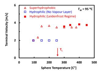
**Figure 4.** Variation of the terminal velocity with the sphere temperature, measured for a 20 mm steel sphere falling through 95 °C water. Open squares (blue) are data for hydrophilic spheres at temperature below the Leidenfrost temperature ( $T_L$  = 260 °C) and solid squares (red) for temperatures above  $T_L$ . Open triangles (red) are data for superhydrophobic spheres (see also Video 1).
