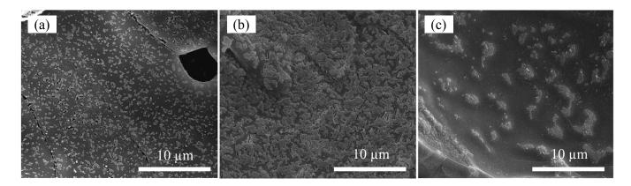
**Figure 12**. Cryo-SEM images of the interface of heptane-in-water (no salt) emulsions stabilised by 0.1 wt.% WPM particles: (a) pH 3 - discrete organisation of individual particles or small aggregates, (b) pH 4.8 - 2-D gel of aggregated particles and (c) pH 7 - flocs of particles.
