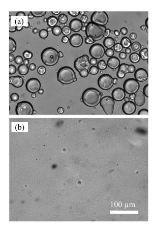
**Figure 1**. Optical microscopy images of a 4 wt.% WPM aqueous dispersion (a) before and (b) after sonication (scale bar is same in both images).
