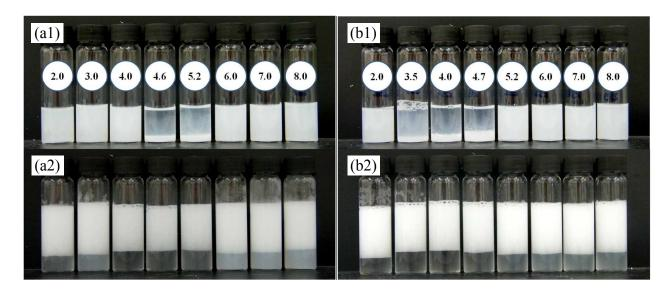
**Figure 4**. (1) Photographs of vessels containing 0.1 wt.% WPM aqueous dispersions and (2) corresponding o/w emulsions (50 vol.% Miglyol 812N) 1 hr. after preparation as a function of pH (given) and salinity; (a) 0 M NaCl, (b) 150 mM NaCl.
