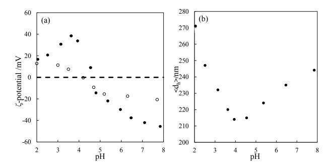
**Figure 6**. Evolution of (a)  $\zeta$ -potential and (b) average hydrodynamic diameter of 0.01 wt.% WPM aqueous dispersions at 25 °C as a function of pH and salinity; filled points 0 M, open points 150 mM NaCl. Note the strong reduction of the  $\zeta$ -potential in the presence of 150 mM due to compression of the electrical double layer at the surface of the WPM.
