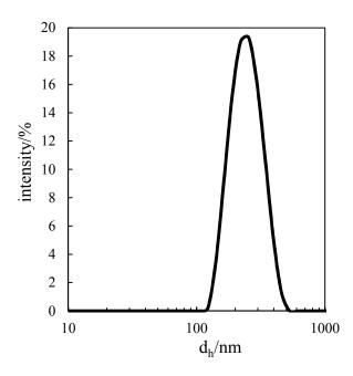
**Figure 2**. Particle size distribution *via* light scattering of a 0.01 wt.% WPM aqueous dispersion at 25 °C and natural pH (6.5).
