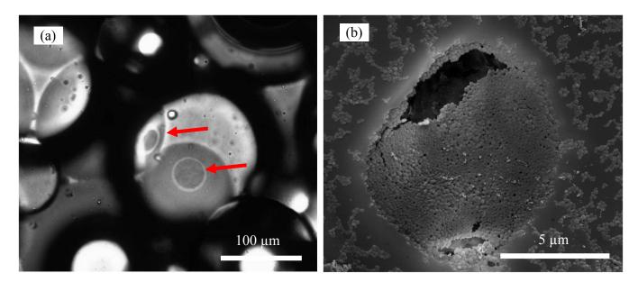
**Figure 14**. (a) Optical microscopy image of flat adhesive films (indicated by red arrows) between flocculated heptane drops in an o/w emulsion stabilised by WPM at pH 6 and (b) cryo-SEM image of a flat adhesive film between two heptane drops in water at pH 6 viewed from above. The contact zone between the drops forms a disc of close packed particles; note the lower concentration of adsorbed particles outside of this zone.
