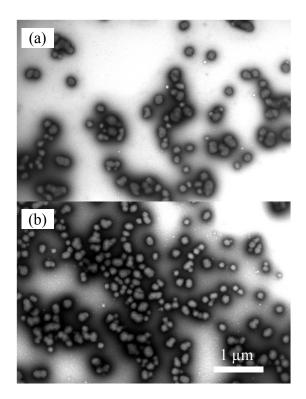
**Figure 3**. Negative-staining TEM micrographs from 4 wt.% WPM aqueous dispersions; (a) freshly prepared (before spray-draying) and (b) after sonication of spray-dried powder.
