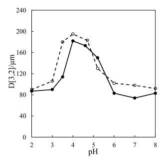
**Figure 8**. Evolution of the average drop diameter of o/w emulsions stabilised by 0.1 wt.% WPM particles as a function of pH; filled points – 0 M NaCl, open points - 150 mM NaCl.
