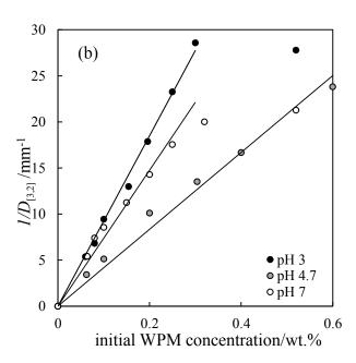
**Figure 10**. Evolution of the inverse of the average drop diameter  $(I/D_{[3,2]})$  for Miglyol 812N-in-water emulsions as a function of the initial WPM particle concentration, c, in the aqueous phase for three different pH; (a) 0 M NaCl, (b) 150 mM NaCl.
