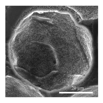
**Figure 11**. Cryo-SEM image of a heptane emulsion drop in water (no salt) covered by 0.1 wt.% WPM particles at pH 3. During fracturing, the frozen oil has been removed allowing direct visualisation of the particles residing at the interface.
