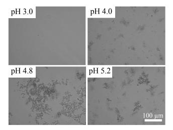
**Figure 5**. Optical microscopy images of 0.1 wt.% WPM aqueous dispersions without salt 1 hr. after pH adjustment and after gentle manual shaking of the vials.
