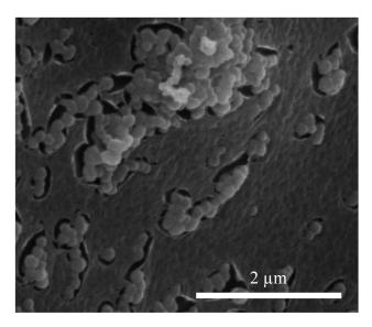
**Figure 13**. Cryo-SEM image of the interface of a heptane-in-water emulsion stabilised by WPM particles at pH 4.8 after light sublimation. The sublimation reveals the presence of a thin film between the particle aggregates.
