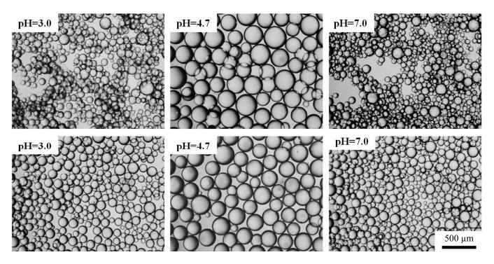
**Figure 7**. Optical microscopy images of o/w emulsions stabilised by 0.1 wt.% WPM particles as a function of pH and salinity; upper row - 0 M NaCl, lower row - 150 mM NaCl.
