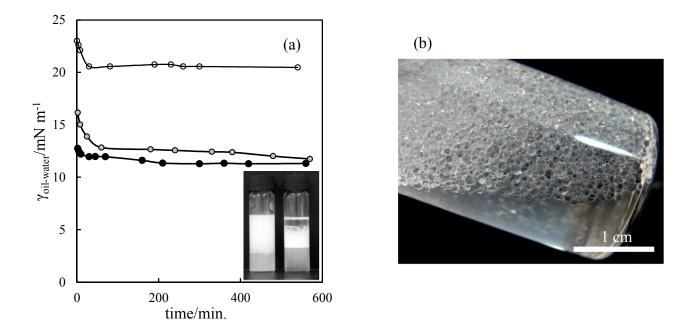
**Figure 15**. (a) Evolution of the Miglyol 812N-water interfacial tension at 25 °C with time for 3 different aqueous phases at pH 7: open circles - pure water, filled circles - 0.1 wt.% WPM, grey circles - filtrate of 0.1 wt.% WPM dispersion. Insert – photo' of emulsions 2 days after preparation stabilised by (left) 0.1 wt.% WPM and (right) the filtrate obtained after filtration of 0.1 wt.% WPM dispersion through a
