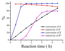
Figure 2. Reaction kinetic plot for the synergistic photocatalytic oxidation of sulfide and amine with O<sub>2</sub> on TiO<sub>2</sub> under visible light irradiation. Reaction conditions: 0.3 mmol of thioanisole 1, 0.1 mmol of benzylamine 2, 40 mg of TiO<sub>2</sub>, 300 W Xe lamp, λ>400 nm, 5 mL of CH<sub>3</sub>OH, 0.1 MPa of O<sub>2</sub>.
