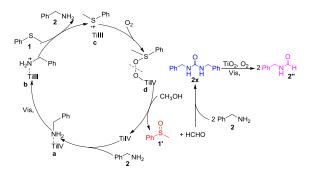
Scheme 1 Proposed mechanism for the synergistic selective oxidation of thioanisole 1 and benzylamine 2 with O<sub>2</sub> on TiO<sub>2</sub> under visible light irradiation.
