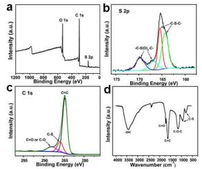
**Fig. 3** XPS (a) S2p (b) C1s (c) and FTIR (d) spectra of S-GQDs. Reprinted with permission from: ref. 20, copyright 2014 American Chemical Society.
