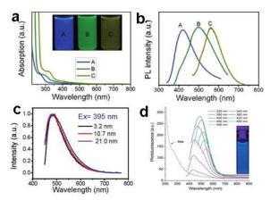
Fig. 4 (a) UV-vis spectra of GQDs A, B, and C, corresponds to synthesized reaction temperature at 120, 100, and 80 °C, respectively. Inset of panel is a photograph of the corresponding GQDs under UV light
