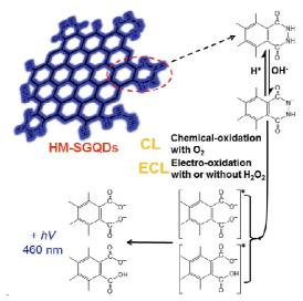
Fig. 13 CL and ECL mechanisms of HM-SGQDs. Reprinted with permission from ref. 85, copyright 2014 Royal Society of Chemistry.
