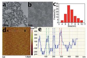
**Fig. 1** TEM (a) and HRTEM (b) images and size distribution (c) of GQDs. (d) AFM image of the GQDs deposited on freshly cleaved micasubstrates. (e) Height profile along the line from A to B in (d). Reprinted with <sup>40</sup> permission from: ref. 33, copyright 2012 Royal Society of Chemistry.
