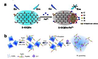
**Fig. 7** (a) Schematic illustration of the PL quenching mechanism of the S-GQDs in the presence of Fe<sup>3+</sup>. (b) Schematic representation of the CK2 <sup>60</sup> kinase assay based on the aggregation and PL quenching of phosphorylated peptide-GQD conjugates *via* Zr<sup>4+</sup> linkages. Reprinted with permission from: (a): ref. 20, copyright 2014 American Chemical Society, (b): ref. 63, copyright 2013 American Chemical Society.
