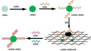
Fig. 9 Schematic illustration of a universal PL sensing platform for the 85 detection of DNA based on LRET between GQDs and GO. Reprinted with permission from ref. 71, copyright 2014 Royal Society of Chemistry.
