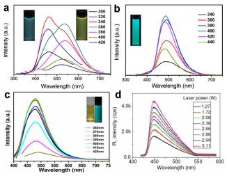
**Fig. 6** PL spectra of the B-GQDs aqueous solution in the absence (a) and <sup>10</sup> presence (b) of borax. (c) PL spectra of S-GQD. (d) Upconversion photoluminescence spectra obtained from GQDs under excitation of a femtosecond pulsed laser at 800 nm. Reprinted with permission from: (a) and (b): ref. 19, copyright 2014 Elsevier, (c): ref. 20, copyright 2014 American Chemical Society, (d): ref. 57, copyright 2013 Wiley-VCH,
