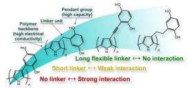
Introducing a linker unit in polypyrrole/quinone conducting redox polymers dramatically reduces the interaction between the two redox systems. Moreover, increasing its length and flexibility completely eliminates the interaction.
