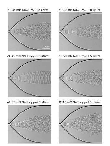
**Fig. 2** Outside of the junction, the droplets were stretched by the surrounding flow and assumed very elongated shapes. At the top of each panel, the salt concentration and the estimated corresponding equilibrium surface tension are reported. The typical production rate is about 200 Hz. The surface tension were interpolated from data in ref. [12].
