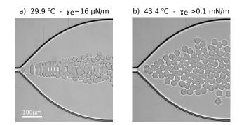
Fig. 3 Droplets at the junction exit with salt concentration of 47.3 mM at temperatures higher than the corresponding PIT, namely 24.3°C. The equilibrium surface tension increased with increasing temperature and for values higher than 0.1mN/m, the droplet population was monodisperse. In panel b), the droplet diameter is  $22.7 \pm 0.8 \,\mu$ m.
