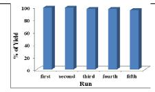
25 Figure 2 Reusability of the heterogeneous PdNPs/TMC catalyst in Suzuki reaction
