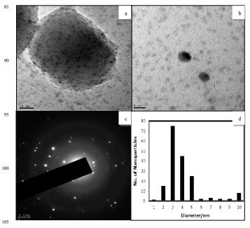
Figure 1. a) TEM image of heterogeneous catalyst PdNPs/TMC b) HR-TEM image of PdNPs/TMC (spherical nanoparticles around 3-5 nm) c) SAED image of PdNPs/TMC catalyst d) Histogram of PdNPs/TMC heterogeneous catalyst.
