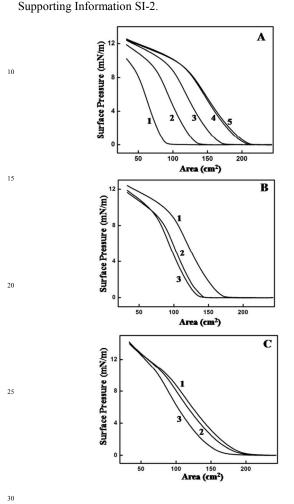
Fig. 1: (A) Surface pressure-area (Π-A) isotherms of CdSe QDs on water subphase by adding successively increased volume: 5, 10, 15, 20 and 25 μl of sample corresponding to the curve numbers 1-5. (B) Π-A isotherms of CdSe QDs with 15 μl of sample at t=10 min (Curve 1), t=90 min 35 (Curve 2) and t=2 h (Curve 3). (C) Π-A isotherms of CdSe QDs with 30 μl of sample at t=10 min (Curve 1), t=90 min (Curve 2) and t=2 h (Curve 3) over HAuCl<sub>4</sub> subphase.
