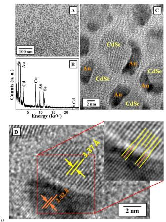
Fig. 4: (A) Transmission electron microscopic image at low magnification for Au-CdSe hybrid formed via LB technique. (B) EDX as obtained from this region of the sample. (C, D) HRTEM image of hybrid nanostructure: the lattice planes of Au and CdSe were clearly visible. 90 Fourier-filtered image in the inset of (D) showed misfit dislocations at the interface.
