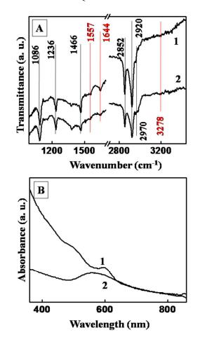
Fig. 2: (A) FTIR spectra of oleyl amine capped CdSe QDs (Curve 1) and 70 oleyl amine capped Au-CdSe hybrid nanocomposite (Curve 2) obtained by depositing the monolayer on Si (111) substrate. (B) UV-Vis-NIR spectra of CdSe QDs (Curve 1) and Au-QD hybrid (Curve 2) obtained by depositing the samples on quartz plate from LB monolayer.
