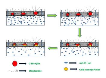
**Scheme 1:** Schematic diagram for plausible mechanism of formation of Au tip selectively at one side of CdSe QD via LB technique.
