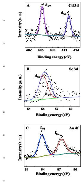
Fig. 3: XPS analysis of CdSe-Au hybrids for (A) Cd 3d, (B) Se 3d and (C) Au 4f.
