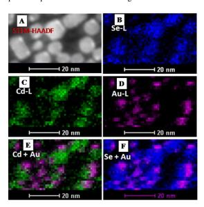
Fig. 5: (A) Scanning TEM-HAADF image of CdSe-Au which was <sup>20</sup> deposited at t=20 min after exposure of CdSe to aqueous HAuCl<sub>4</sub> subphase. (B-D) EDX maps obtained from same area in A using Se L, Cd L and Au L energy, respectively of the representative elements in Au-CdSe. (E, F) Overlay of Cd - Au and Se - Au.
