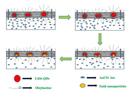
Oleyl amine capped CdSe quantum dots are allowed to form monolayer on aqueous  $HAuCl_4$  subphase and Langmuir-Blodgett technique is used judicially to grow Au tips in a directed fashion on CdSe quantum dots.
