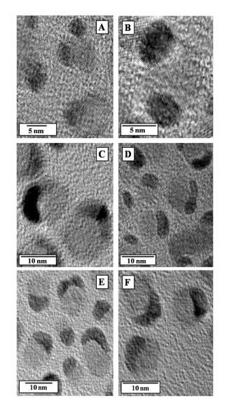
**Fig. 6: (A-F)** Transmission electron microscopic images taken after spreading the QDs on HAuCl<sub>4</sub> subphase in LB trough for t=2 min, 5 min, 10 min, 15 min, 20 min and 90 min respectively
