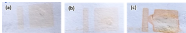
Figure 11. Photographs of printed solid forms on cellulose substrates after irradiation and rinsing steps: (a) 1-pass printing, (b) 3-pass printing and (c) 6-pass printing.
