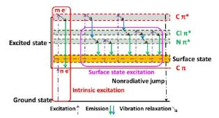
Figure 3 Diagram of energy levels and the electronic transitions in the GQDs
