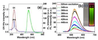
**Figure 2** (a) UV-Vis spectrum (blue line) and FL spectra (red and green lines) of obtained GQDs; (b) Typical FL spectra of obtained GQDs, and photos of the GQDs solution under visible (left) and 365 nm UV (right) light
