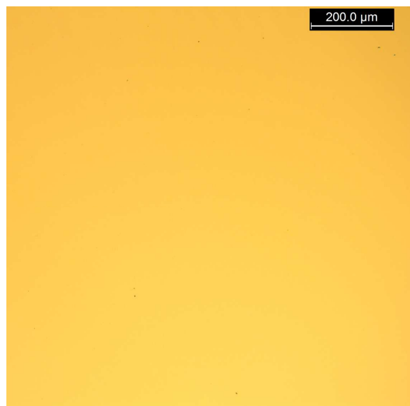
Fig. S2 Optical image of 1 mm 2 area EPD ZnO film obtained at 5V for 120 s.
