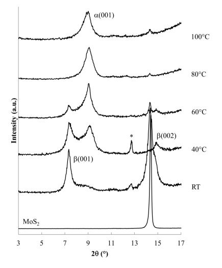
Figure 3. Powder XRD of  $MoS_2$  and the intercalation compounds obtained after 24 h at reaction temperatures ambient to 100°C.
