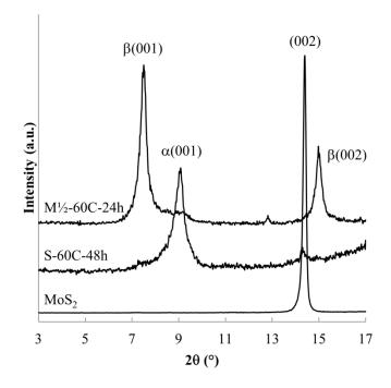
Figure 2. Powder XRD of MoS<sub>2</sub> and the intercalation compounds obtained after 48 h reaction at 60°C (S-60C-48h) and after 24 h reaction at 60°C using decreased Na mass (M<sup>1</sup>/<sub>2</sub>-60C-24h).
