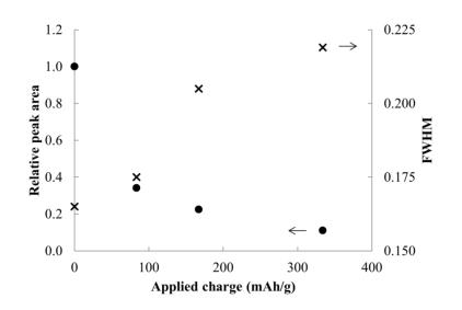
Figure 12. Relative peak areas and widths for MoS<sub>2</sub> and reduction products at different applied charges.
