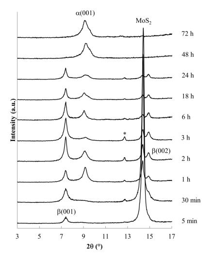
Figure 4. Powder XRD data obtained for reaction of  $MoS_2$  with Na/en electride solution at 60°C. Reaction times are indicated at the right.
