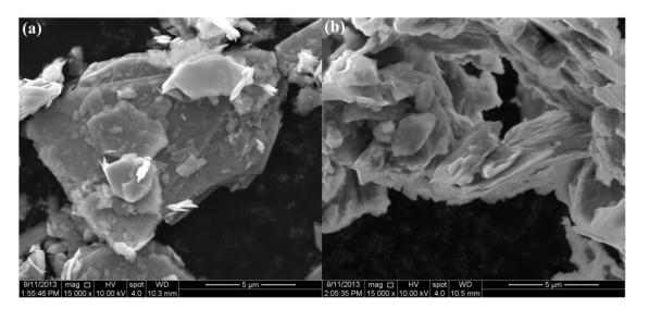
Figure 9. SEM images of (a)  $MoS_2$  and (b)  $\alpha$  phase intercalation compound  $Na_{0.3}MoS_2$ ·0.4en
