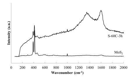
Figure 10. Raman spectra of  $MoS_2$  and Na-en- $MoS_2$  intercalation compound (S-60C-3h) indicates the structural change upon intercalation.
