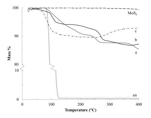
Figure 8. Thermograms of  $MoS_2$ , en, (a) the  $\alpha$  phase Na-en-MoS<sub>2</sub> intercalation compound (S-60C-48h) and (b) a  $\beta$  phase predominant product (S-60C-3h) under Ar flow, and (c)  $\beta$  phase predominant product (S-60C-3h) analyzed under air flow.
