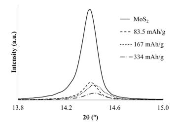
Figure 11. Powder XRD profiles for  $MoS_2$  and products of electrochemical reduction in  $en/NaPF_6$  with applied charges indicated.
