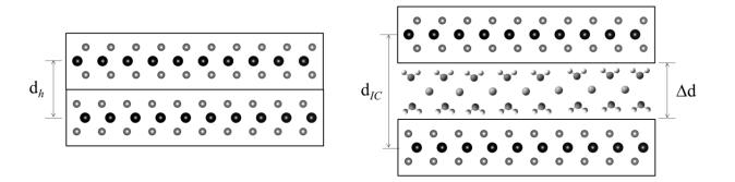
Figure 1: Schematic representations of  $MoS_2$  and  $Na_xMoS_2 \cdot \delta H_2O$ , where  $H_2O$  is a cointercalate.
