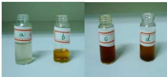
Fig. 4 Test for the production of hydrogen peroxide in the reaction mixture of 1a and 2a . (a) KI and starch in glacial acetic acid, colourless. (b) The reaction mixture of 1a and 2a after reaction completed, brown. (c) Addition of solution (b) to solution (a), dark red. (d) Addition of 30% of H_2O_2 in solution (a). KI (0.2 M), aqueous acetic acid (0.2 M), starch (4 mg/mL), DPZ H (0.1 \mu mol, 14.14 \mu L, 2.5 mg/mL in CH_3NO_2 ), 1a (0.1 mmol), CH_3NO_2 (1.0 mL), reaction time: 5 h, 28 ^{\circ}C .
