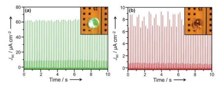
**Figure 86**: Rectified Jsc of the as-developed TENG before (a) and after (b) the interaction with 5  $\mu$ M Hg<sup>2+</sup> ions. Insets: photograph of the indicated LED lamp before (a) and after (b) interaction with 5  $\mu$ M Hg<sup>2+</sup> ions, as an indication of detected concentration. Reprinted with permission from ref 129. Copyright 2013 Wiley.
