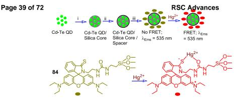
**Figure 45.** Strategy used for FRET base Hg<sup>2+</sup> sensor on QDs.
