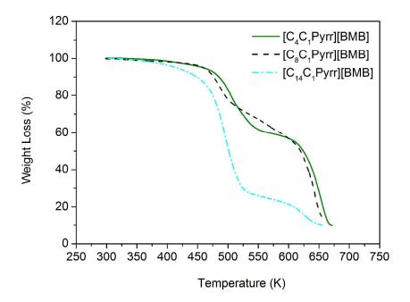
**Figure 3.** Thermogravimetric analysis of *N*-alkyl-*N*-methylpyrrolidinium bis(mandelato)borate hf-BILs.
