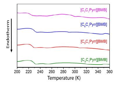
**Figure 1.** DSC thermograms of selected *N*-alkyl-*N*-methylpyrrolidinium bis(mandelato)borate hf-BILs.
