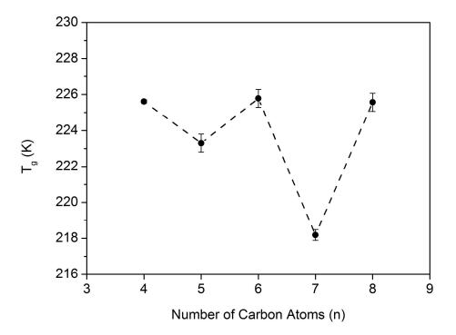
**Figure 2.** "Odd-even" effect of the longest alkyl chain length in N-alkyl-N-methylpyrrolidinium bis(mandelato)borate on the glass transition temperature ( $T_g$ ).
