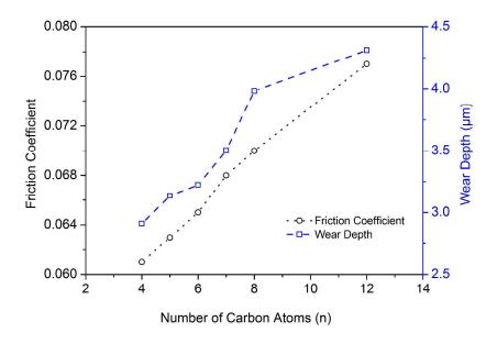
**Figure 8.** The effect of the alkyl chain length of *N*-alkyl-*N*-methylpyrrolidinium bis(mandelato)borate on the wear depth and friction coefficient. The tests were
