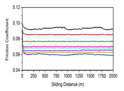
**Figure 6.** Variation of the friction coefficient with the sliding distance in the steel ball on steel disk contact lubricated by 5W40 oil, neat PEG or PEG with 3 wt% [C<sub>n</sub>C<sub>1</sub>Pyrr][BMB]. Room temperature (298 K), 15N load, 0.2 m/s sliding speed. Friction curves from top to bottom: 5W40, neat PEG, [C<sub>12</sub>C<sub>1</sub>Pyrr][BMB]/PEG,
