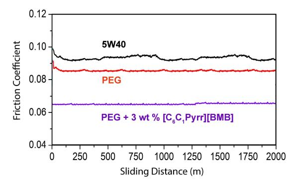
Friction coefficients for a pyrrolidinium orthoborate ionic liquid as 3 wt% additive in PEG, neat PEG and 5W40.
