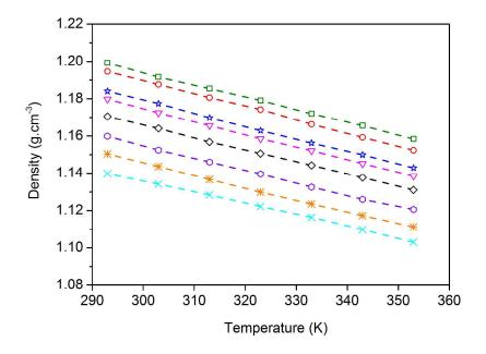
**Figure 4.** Density of *N*-alkyl-*N*-methylpyrrolidinium bis(mandelato)borate hf-BILs as a function of temperature. From top to bottom:  $[C_4C_1Pyrr][BMB]$ ,  $[C_5C_1Pyrr][BMB]$ ,  $[C_6C_1Pyrr][BMB]$ ,  $[C_7C_1Pyrr][BMB]$ ,  $[C_8C_1Pyrr][BMB]$ ,  $[C_{10}C_1Pyrr][BMB]$ ,  $[C_{12}C_1Pyrr][BMB]$  and  $[C_{14}C_1Pyrr][BMB]$ .
