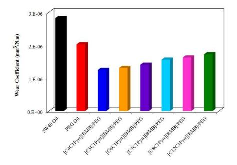
**Figure 7.** Wear coefficients for the discs lubricated by 5W40 oil, neat PEG or PEG containing 3 wt% of a hf-BIL. Tests were performed at room temperature, steel-steel contacts, 15 N load, 0.2 m/s sliding speed.
