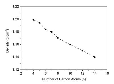
**Figure 5.** Effect of the alkyl chain length of *N*-alkyl-*N*-methylpyrrolidinium bis(mandelato)borate on densities of BILs at 293 K.
