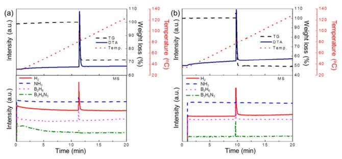
**Fig. 4** TG-DTA-MS profiles of hand-milled AB-MAlH<sub>4</sub> mixtures; (a) AB-NaAlH<sub>4</sub> mixture, (b) AB-LiAlH<sub>4</sub> mixture. The heating rate was 5  $^{\circ}$ C min<sup>-1</sup>.
