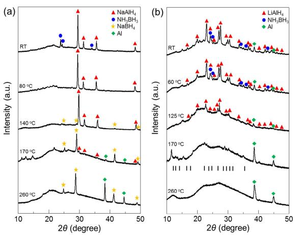
Fig. 2 XRD profiles of ball-milled AB-MAlH<sub>4</sub> composites after heating to each temperature; (a) AB-NaAlH<sub>4</sub> composite, (b) AB-LiAlH<sub>4</sub> composite.
