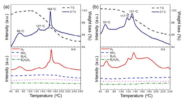
Fig. 1 TG-DTA-MS profiles of ball-milled AB-MAlH<sub>4</sub> composites; (a) AB-NaAlH<sub>4</sub> composite, (b) AB-LiAlH<sub>4</sub> composite. The heating rate was 5 °C min<sup>-1</sup>.
