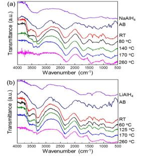
**Fig. 3** *In-situ* FTIR spectra of ball-milled AB-MAIH<sub>4</sub> composites at each temperature; (a) AB-NaAIH<sub>4</sub> composite, (b) AB-LiAlH<sub>4</sub> composite. AB and MAIH<sub>4</sub> (M = Na, Li) spectra was presented for comparison. The heating rate was 5 °C min<sup>-1</sup>.
