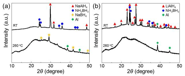
**Fig. 5** XRD profiles of hand-milled AB-MAlH<sub>4</sub> mixtures at RT and after heating to 260 °C; (a) AB-NaAlH<sub>4</sub> mixture, (b) AB-LiAlH<sub>4</sub> mixture.
