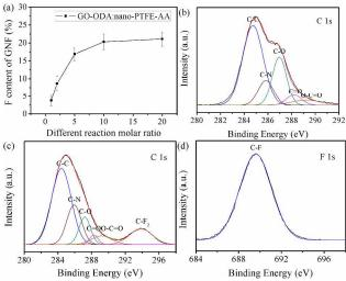
Fig. 2 (a) Relationship of F content of GNF with different reaction molar ratio. C 1s XPS spectra of (b) GO-ODA and (c) GNF, and F 1s XPS spectrum of (d) GNF.
