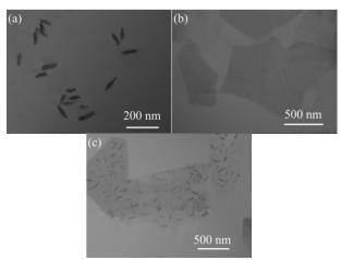
Fig. 4 TEM images of (a) nano-PTFE-AA. (b) GO-ODA and (c) GNF.
