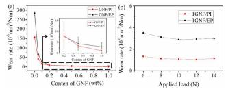
Fig. 6 (a) Relationship of wear rate of GNF/PI and GNF/EP specimens with different GNF content. The inset shows its 25 corresponding enlarged view. (reciprocating frequency: 10 Hz, sliding distance: 480 m, load: 10 N, RH: 40%). (b) Relationship of wear rate of 1GNF/PI and 1GNF/EP specimens with different applied load (reciprocating frequency: 10 Hz, sliding distance: 480 m, RH: 40%).
