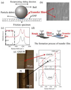
Fig. 10 (a) A schematic for tribological mechanism of GNF/polymer composites. (b) SEM image of transfer film on the counterpart. (c) Raman spectral comparison between transfer film and GNF. (d) The formation process of transfer film. (e) Raman 10 analysis of worn surface of GNF/PI and PI specimens after washing.
