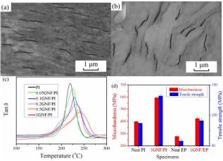
Fig. 8 TEM images showing GNF dispersion of (a) 1GNF/PI and 15 (b) 1GNF/EP specimens. (c) Damping spectra of PI and GNF/PI composites films. (d) Microhardness and tensile strength of neat PI, 1GNF/PI, neat EP and 1GNF/EP specimens.
