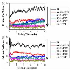
Fig. 5 Friction coefficient values for the (a) GNF/PI and (b) GNF/EP specimens as a function of sliding time. (reciprocating frequency: 10 Hz, sliding distance: 480 m, load: 10 N, RH: 40%)
