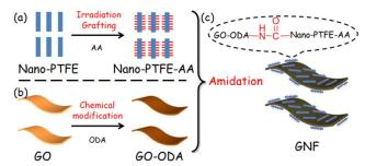
55 Fig. 1 Covalent compounding between GO and nano-PTFE including (a) irradiation grafting of nano-PTFE with AA, (b) chemical modification of GO with ODA and (c) preparation of GNF by amidation reaction between GO-ODA and nano-PTFE-AA.
