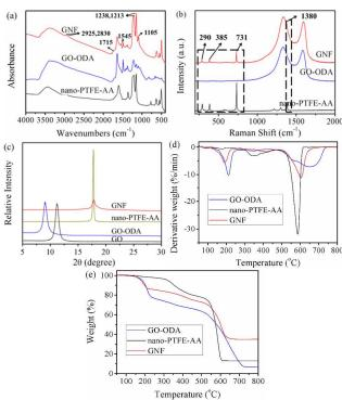
Fig. 3 (a) FTIR spectra, (b) Raman spectra (excitation 65 wavelength 631 nm), (c) XRD patterns, (d) DTG curves and (e) TGA thermograms of nano-PTFE-AA, GO-ODA and GNF.
