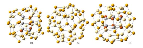
**Figure 2.** The (a)  $(CdSe)_{33}$ , and (b), (c)  $(CdSe)_{34}$  cage clusters. For (a) and (c) the internal cages have been highlighted for clarity. (b) The orientation is along the main axis of symmetry.
