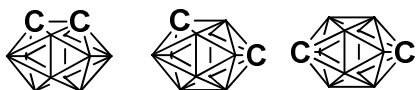
Figure 1. Structures of (left-right): ortho -carborane, meta -carborane and para -carborane. Unlabelled vertices represent BH units. Protons omitted for clarity.
