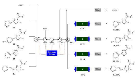
Scheme 6 Automated oxidation of oxazolines using a Raspberry Pi® computer and a multiple position valve.
