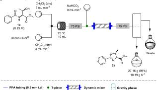
Scheme 3 Platform set up for the scale up experiment.
