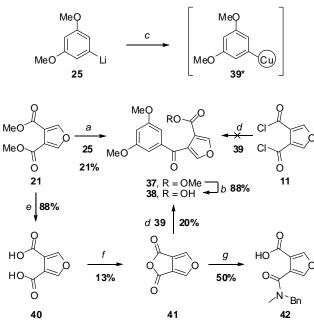
Scheme 6. Reagents and conditions: (a) THF,  $-78 \ ^{\circ}C \rightarrow RT$  (product is 37); (b) LiOH, MeOH/H<sub>2</sub>O, 0  $\ ^{\circ}C$ ; (c) CuCN.2LiCl, THF,  $-78 \rightarrow -40 \ ^{\circ}C$ , \*The structure of such organocuprates is poorly understood; (d) THF,  $-78 \ ^{\circ}C \rightarrow RT$ , 2. H<sub>3</sub>O<sup>+</sup> (product is 38); (e)<sup>19</sup> 1. 20% NaOH, reflux, 2. H<sub>3</sub>O<sup>+</sup>; (f) Ac2O, reflux; (g) xs BnNHMe, DCM.
