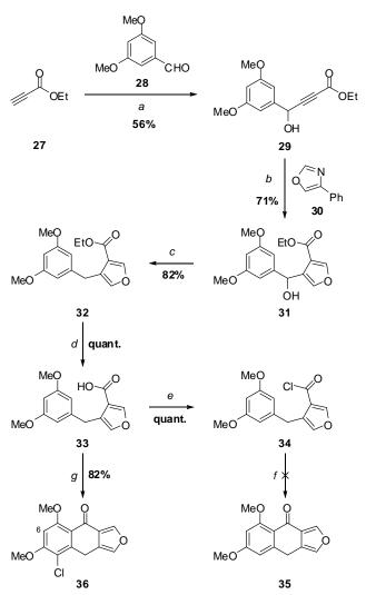
Scheme 5. Reagents and conditions: (a) 1. BuLi, THF,  $-100 \,^{\circ}$ C, 2. 28; (b) hydroquinone, 200  $^{\circ}$ C; (c) TMSCl, NaI, MeCN; (d) 1. NaOH, MeOH, 2. H<sub>3</sub>O<sup>+</sup>; (e) (COCl)<sub>2</sub>, 0  $^{\circ}$ C (crude yield indicated); (f) AlCl<sub>3</sub>, DCE, 0  $^{\circ}$ C or <sup>5</sup> SnCl<sub>4</sub>, PhH, 0  $^{\circ}$ C; (g) 1. PCl<sub>5</sub>, PhH, reflux, 2. SnCl<sub>4</sub>, 0  $^{\circ}$ C.
