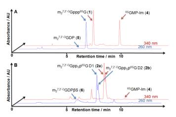
Fig. 2. RP HPLC profiles from the synthesis of cap analog 1 (A) and diastereomeric mixture of 2a and 2b (B)
