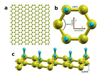
Fig. 1 Configurations of graphone. a graphone plane; b top-view and directions; c side-view.
