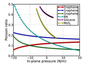
Fig. 4 Pressure effect on the Poisson ratio. The Poisson ratio as a function of the pressure of graphone is peculiar compared to those of other two-dimensional structures including graphene<sup>26</sup>, graphane<sup>26</sup>, *h*-BN monolayer<sup>25</sup>, silicene<sup>33</sup>, and MoS<sub>2</sub> monolayers<sup>34</sup>.
