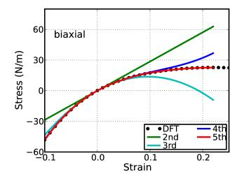
**Fig. 3 Limits of higher order effects.** Predicted stress-strain responses of biaxial deformation of graphone from different orders of elastic constants compared to that from the density functional theory (DFT) calculations (dotted line) indicates the limitations are 0.02, 0.07, 0.14, and 0.22 for second, third, fourth, and fifth order elastics, respectively.
