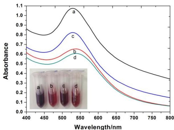
**Fig. 2** Absorption spectra and photographs (inset) of solution: (a) Tween 80 + HAuCl<sub>4</sub> (b) Tween 80 + HAuCl<sub>4</sub> + lipase (c) Tween 80 + HAuCl<sub>4</sub> + 1 mM oleic acid (d) Tween 80 + HAuCl<sub>4</sub> + 2 mM oleic acid.
