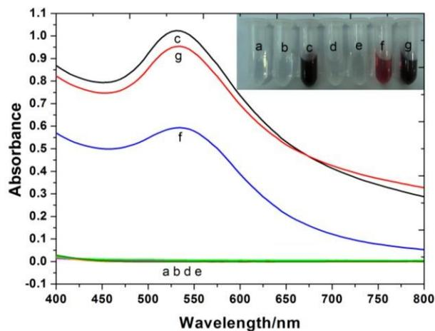
**Fig. 1** Absorption spectra and photographs (inset) of solution: (a) Tween 80 (b) HAuCl<sub>4</sub> (c) Tween 80 + HAuCl<sub>4</sub> (d) Tween 80 + lipase (e) HAuCl<sub>4</sub> + lipase (f) Tween 80 + HAuCl<sub>4</sub> + lipase (g) Tween 80 + HAuCl<sub>4</sub> + inactivated lipase.
