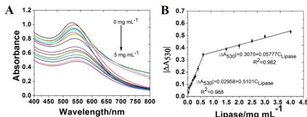
**Fig. 6** (A) Absorption spectra of different concentrations of lipase; (B) calibration curves.
