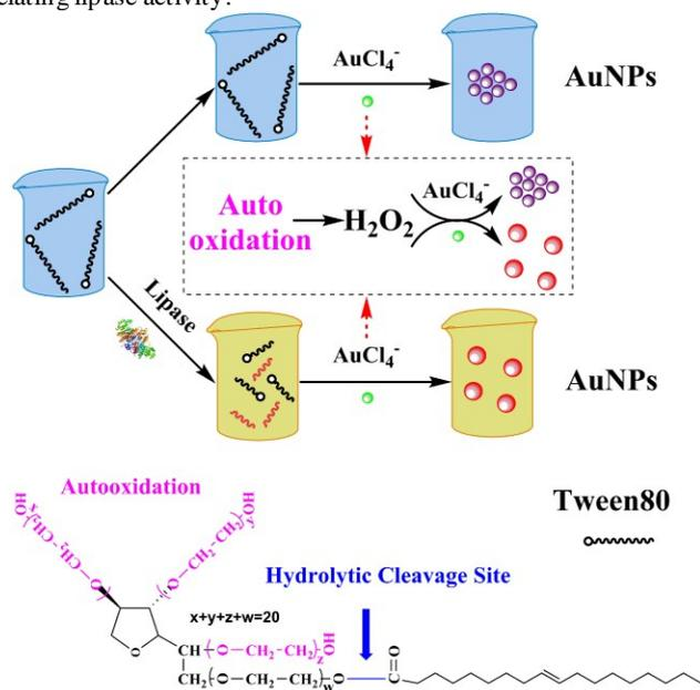
**Scheme 1** Schematic illustration of the colorimetric lipase assay based on enzyme-controlled AuNPs growth *in situ*.
