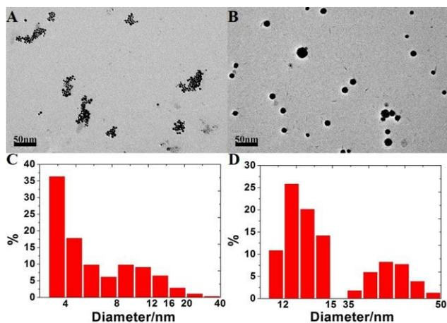
**Fig. 3** TEM images: (A) AuNPs; (B) AuNPs + lipase; Particle size distribution (C) AuNPs, (D) AuNPs + lipase
