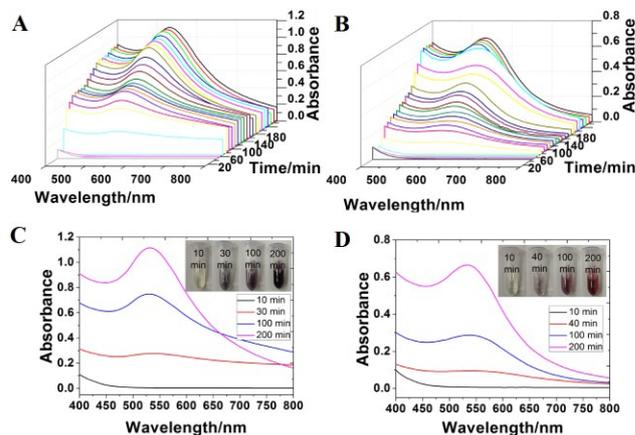
**Fig. 4** *In situ* absorption spectra recording the growth process of the AuNPs (A) in the absence of lipase (B) in the presence of lipase. (time interval : 10 min.) Absorption spectra and the corresponding photographs (inset) of AuNPs obtained in different time interval (C) in the absence of lipase (D) in the presence of lipase.
