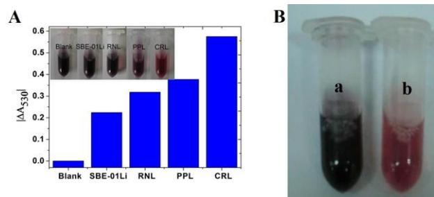
**Fig. 7** (A) The plot of  $|\Delta A_{530}|$  values of the formed AuNPs, inset: the corresponding photographs; (B) Photographs of the formed AuNPs upon adding (a) inactivated and (b) activated fermentation broth of *Bacillus subtilis*.
