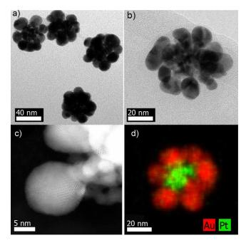
Fig. 3 a) TEM image of typical Pt@Au core-satellite particles, b) HRTEM image of a single Pt@Au core-satellite NP, c) High resolution HAADF-STEM image of a single Au 'petal' located around the Pt dendrite core. Twinning is observed. d) EDX map of a Pt@Au coresatellite particle.
