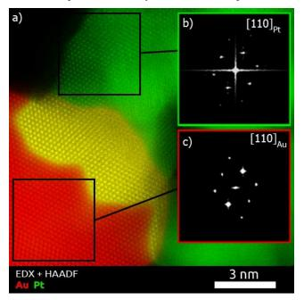
**Fig. 2** a) EDX map overlaid to the corresponding high resolution HAADF-STEM image of the Au-Pt interface in a dimer. b,c) FFT patterns from the highlighted regions, showing the [110] zone axis of the fcc crystal structure.
