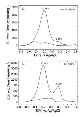
Fig 5. Cyclic voltammograms recorded at GC-Pt-Au (a) and GC-Pt@Au (b) in 1 M ethanol and 1 M NaOH aqueous solution. The scan rate was  $50 \text{ mVs}^{-1}$ .
