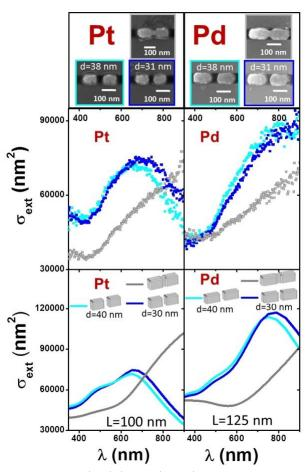
Figure 7: Experimental and theoretical optical extinction cross-sections and corresponding SEM images of Pt and Pd dimers for two different interparticle distances and for two touching parallelepipeds of total length equal to that of the non-touching dimers with the interparticle distance included. In calculations the NAs are assumed to be embedded in a homogeneous medium of optical index  $n_{ext}$ =1.25.
