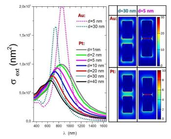
Figure 8: (left) Calculated extinction cross-sections of platinum and gold parallelepipedal dimers (L=100 nm, w=60 nm, h=70 nm) for several interparticle distances. (right) Cross-section views of the EM field magnitude (for the wavelength corresponding to the LSPR maximum) in the plane corresponding to the bottom of the NAs for two interparticle distances (d=5 nm and d=30 nm). The NAs are assumed embedded in a homogeneous medium of optical index n<sub>ext</sub>=1.25.
