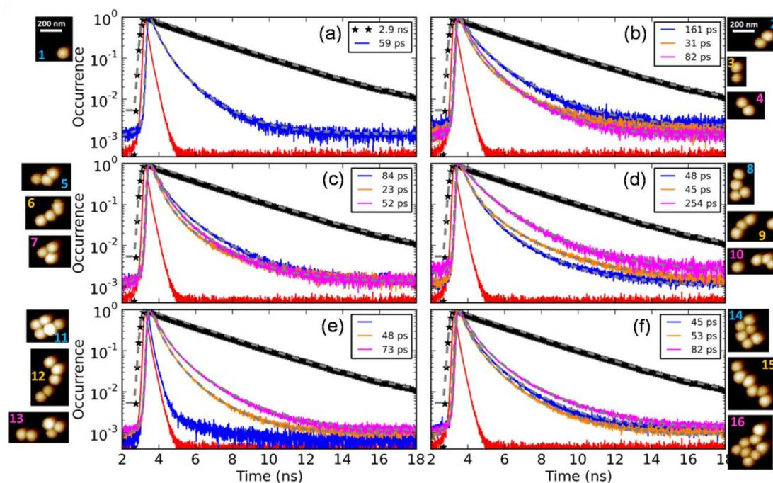
**Fig. 7** Fluorescence decay curves of Rhodamine B on the Au@SiO<sub>2</sub>@Rhodamine B NP oligomers shown in the AFM images next to each panel. The black curve corresponds to isolated Rhodamine B molecules in solution. Values of the estimated decay times are given in the legends. For each panel, the AFM images and legend information are correlated by their vertical positions and colour code.
