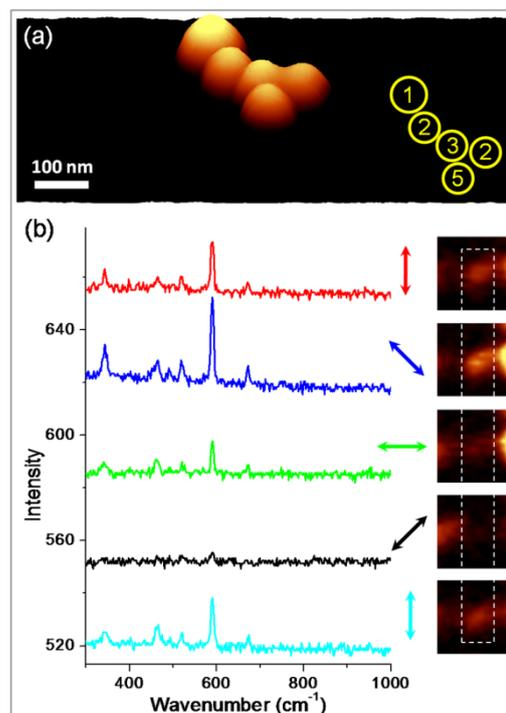
**Fig. 5** (a) AFM 3D image of a Au@TDSP NP pentamer; inset schematizes the structure used for FDTD simulations; (b) SERS spectra and images (inset) of Cresyl Violet on this NP pentamer, for the incident polarizations indicated by arrows.
