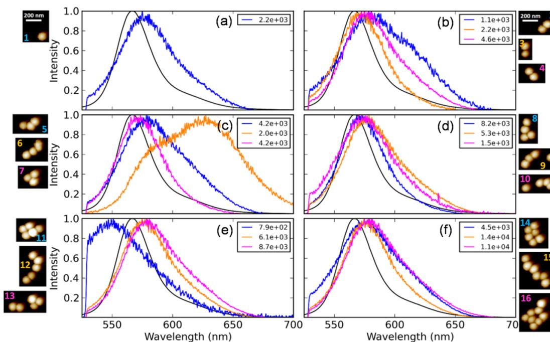
**Fig. 9** Emission spectra (normalized) of the Au@SiO<sub>2</sub>@Rhodamine B NP oligomers shown in the AFM images next to each panel. The black curve corresponds to the emission of isolated Rhodamine B molecules in solution. Values of the maximum emission intensity are given in the legend. Note that these spectra correspond to the decay curves in Figure 7. For each panel, the AFM images and legend information are correlated by their vertical positions and colour code.
