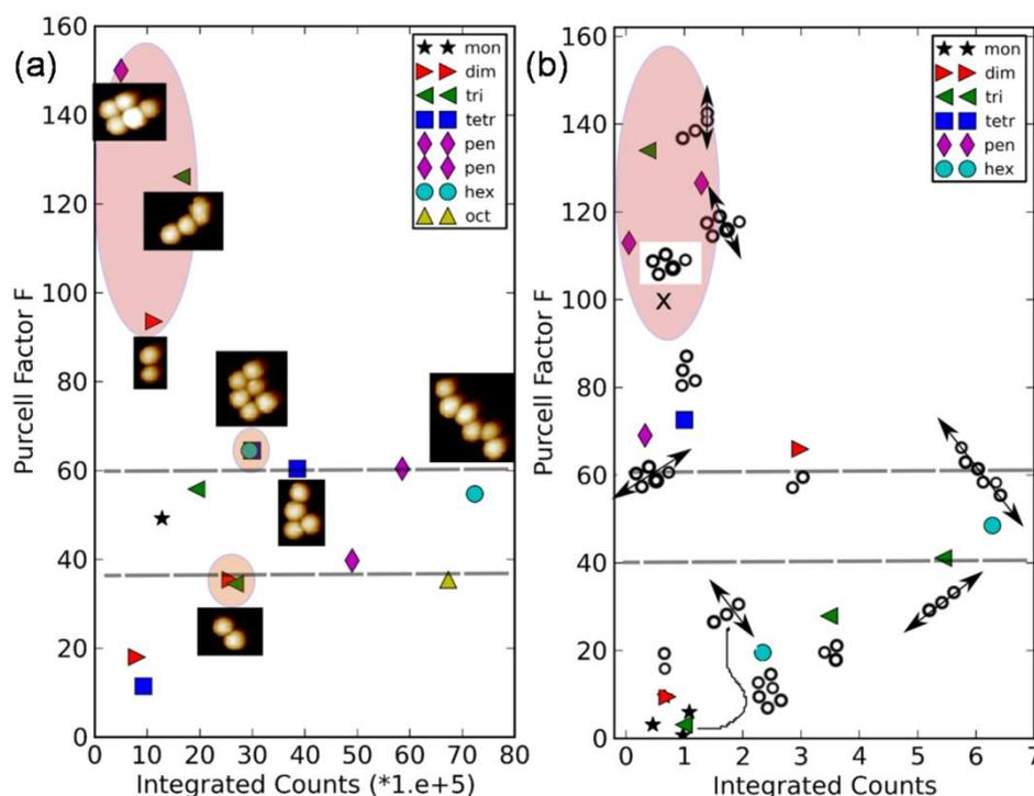
**Fig. 8** Correlation plot between the Purcell factor and integrated emission intensity obtained by experiment (a) and simulations (b) on different Au@SiO<sub>2</sub>@RhodamineB NP oligomers.
