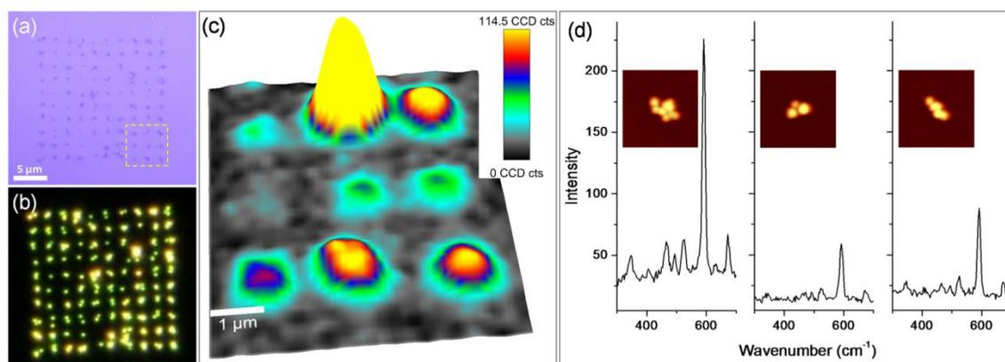
**Fig. 3** (a) Bright-field and (b) dark-field optical microscopy images of an array of  $10 \times 10$  Au@TDSP NP oligomers assembled on charge dots written with +60 V voltage pulses, using a colloidal suspension of concentration  $C_0 = 6 \times 10^{10}$  NPs/mL. (c) SERS image of the area marked in a), constructed from the Cresyl Violet  $589 \text{ cm}^{-1}$  SERS band intensity; (d) selection of SERS spectra with corresponding sites in the inset. Caption
