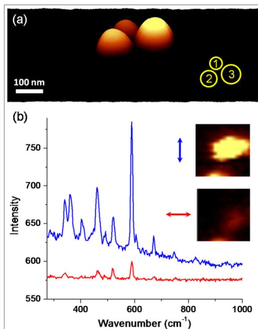
**Fig. 4** (a) AFM 3D image of a NP trimer; inset schematizes the structure used for FDTD simulations. (b) SERS spectra and images (inset) of Cresyl Violet on this NP trimer, for the two incident polarizations indicated by arrows.
