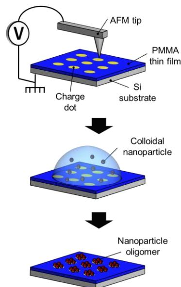
**Fig. 1** Schematics of AFM nanoxerography: AFM charge writing (top), development by incubation of the colloidal suspension on the charge patterns (middle), and resulting nanoparticle oligomer array (bottom).
