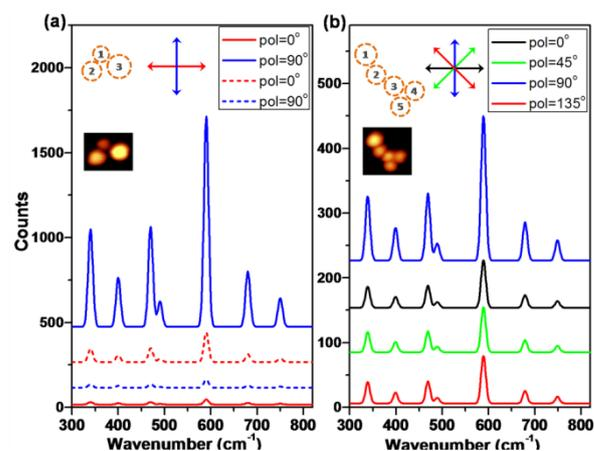
**Fig. 6** Simulated enhanced Raman spectra of: (a) the Au@TDSP NP trimer, for the two indicated incident polarizations, with the emitter located in the gap between particles 1 and 2 (solid lines), and between particles 1 and 3 (dash lines); (b) the Au@TDSP pentamer, for multiple polarizations as indicated, with the emitter located in the gap between particles 3 and 4.
