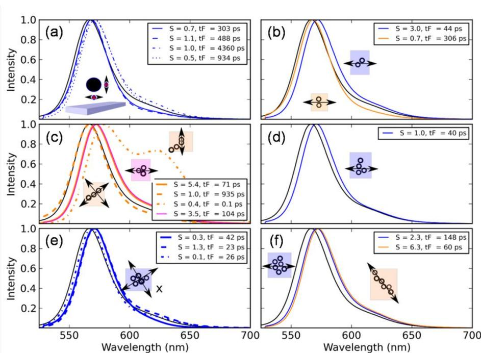
**Fig. 10** Simulated emission spectra (normalized) for the indicated oligomer configurations. Insets report values of the total integrated spectrum and decay time.
