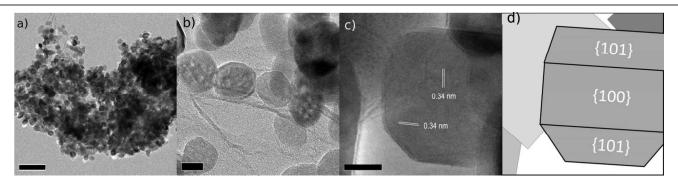
Figure 11: TEM micrographs of GNP—TiO<sub>2</sub>: a) and b) low magnification, c) high resolution showing the 0.34 nm spacing among crystal planes, indicative of the with anatase {101} (trapezoidal) and {100} (rectangular) facets, as shown in d). Scale bars are 200 nm on a), 20 nm on b) and 10 nm on c.
