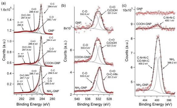
Figure 2: High resolution XPS spectra for GNP, NH<sub>2</sub>–GNP and COOH–GNP samples relative to C 1s (a), O 1s (b) and N 1s (c)
