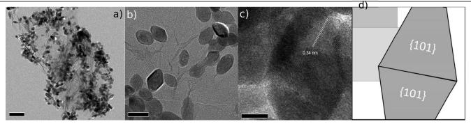
Figure 9: TEM micrographs related to COOH-GNP-TiO<sub>2</sub>: a) and b) low magnification micrographs, c) high magnification micrograph. The o.34 nm spacing shown in c) identifies the two trapezoidal facets as anatase {101} facets; d), schematic of c). Scale bars are 200 nm on a), 50 nm on b) and 10 nm on c).
