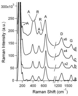
Figure 7: Raman spectra of COOH–GNP–TiO<sub>2</sub> (a), NH<sub>2</sub>–GNP–TiO<sub>2</sub> (b) and of bare GNP–TiO<sub>2</sub> sample taken in different spots (c,d). The label A stands for anatase, R for rutile, D for graphene D peak and G for graphene G peak
