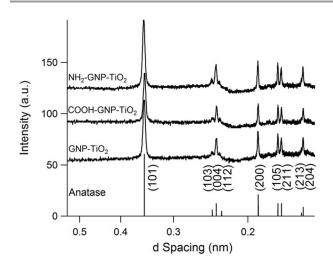
Figure 8: X-ray diffractograms of the GNP- $TiO_2$  hybrids and the reference pattern for anatase (JCPDS No.21.1272)
