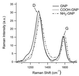
Figure 4: Raman spectra of bare GNP and COOH and  $NH_2$  functionalized GNPs in the 1000–1700 cm $^{-1}$  range. Spectra are normalized with respect to the G peak, the label D stands for for graphene D peak and G for graphene G peak
