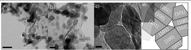
Figure 10: TEM micrographs of NH<sub>2</sub>-GNP-TiO<sub>2</sub> sample: a) and b) low magnification, c) high magnification showing belted bipyramid TiO<sub>2</sub> nanoparticles. The detectable line spacing is around 0.34 nm (Fig. S5). These values indicate the presence of the anatase {101} and {100} surfaces, as shown in d), schematic of c). Scale bars are 200 nm on a), 50 nm on b) and 10 nm on c.
