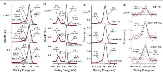
Figure 6: High resolution XPS spectra for GNP-TiO2, NH2-GNP-TiO2 and COOH-GNP-TiO2 samples relative to C 1s (a), Ti  $2p_{1/2}$  and Ti  $2p_{3/2}$  (b), O 1s (c), and N 1s (c)
