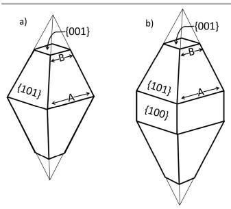
Figure 1: a) Anatase tetragonal bipyramid with eight equivalent  $\{101\}$  surfaces; the truncation gives rise to two equivalent  $\{001\}$  facets; b) Anatase tetragonal belted bipyramid with eight equivalent  $\{101\}$  surfaces, four equivalent  $\{100\}$  facets and, when truncated, two equivalent  $\{001\}$  surfaces. In both a) and b) the degree of truncation is defined as B A $^{-1}$  with 0 < B < A
