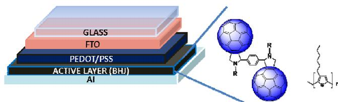
Figure 6. Schematic Illustration of Bulk Heterojunction Organic Photovoltaic Devices prepared with [60] and [70]fullerene homodimers (**4a-c**, **5a-c**), [60]/[70]heterodimer (**6**) and P3HT.
