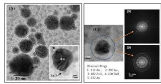
Figure 4: (A) HRTEM image of the nanostructures obtained under magnification. In the expanded view, inset (B), the contact between ZnO and Au is clearly discernible. Panels (D) shows the periodicity of image C by the FFT (Fast Fourier Transform) spectra calculated with the Digital Micrograph software. The same rings were clearly distinguished in the electron diffraction pattern of the Au/ZnO nanostructures.
