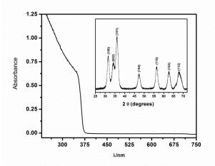
**Figure 1**: UV-Vis spectra of ZnO nanoparticles dispersed in ethylene glycol. Inset XRD pattern of powders obtained by ultracentrifugation of the as-prepared ZnO sol, The peaks corresponding to the reflection from the crystal planes of ZnO are indicated between brackets.
