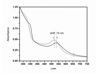
Figure 5: UV-Vis spectra of the Au/ZnO nanostructures obtained before (solid line ) and after (dashed line) anaerobic,  $303 \pm 10$  nm irradiation.
