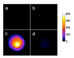
**Fig. 8** False colored pixel intensity maps of a vial containing a solution of chemiluminescent **5EP** (200  $\mu$ L, 1.5 mM in C<sub>2</sub>D<sub>2</sub>Cl<sub>4</sub>) warmed to 38 °C. Emission is only observed using the 695–770 nm filter and not in the other three channels, (a) 515–575 nm, (b) 575–650 nm, or (d) 810–875 nm.
