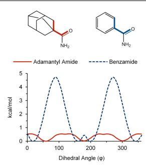
**Fig. 5** Calculated energies for fixed dihedral angles show that the rotation barriers in the adamantyl amide model system are much lower than in the benzamide model system.
