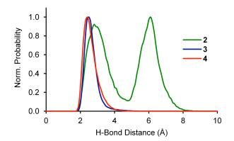
**Fig. 4** Normalized histogram of the distance *d* in the MD simulations 35 of phenylene-sidewall SR 2-4. Two distinct populations are observed for SR 2, but only a single population exists for 3 and 4.
