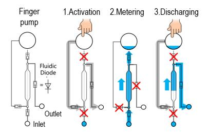
**Figure 2**. The operation and procedural details of the finger-driven MaD. The MaD operation is accomplished using two sequential finger compressions in three steps.
