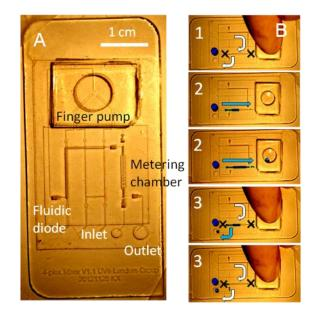
**Figure 4**. The MaD process in a finger-driven microfluidic chip. (A) The chip and labeling of the fluidic components. (B) stepwise snap shots of the MaD process.
