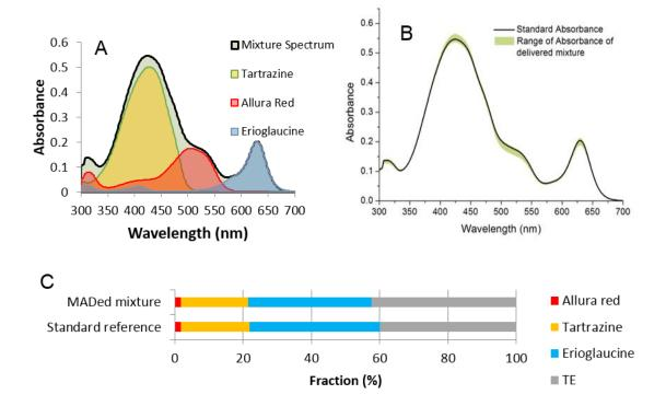
**Figure 7**. The accuracy of finger-driven multi-reagent MaD process. (A) The spectra of the reference mixture containing three different dye solutions at the desired ratio. (B) The comparison between the spectrum of reference mixture and the on-chip metered and delivered mixture with the range shown in green (n=3); (C) Comparison between the ratio of components in the MaD-ed mixture and standard reference
