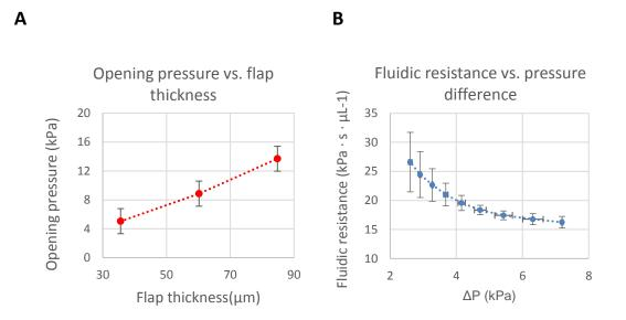
**Figure 3**. Characteristic of the fluidic diode. (A) Open pressure of fluidic diode at forward direction versus flap thickness. (n=3) (B) Relationship between fluidic resistance and pressure difference across the fluidic diode. (n=4)
