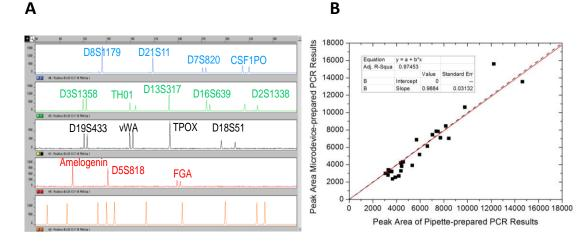
**Figure 9.** PCR results prepared by finger driven microdevice. (A) The electrophoretic STR profile of standard female DNA showing all 16 loci. The reaction mixture was prepared by the finger-driven microdevice; (B) Correlation of peak areas between pipetting-prepared STR-PCR (X-axis) and microdevice-prepared PCR (Y-axis)
