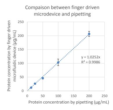
**Figure 8**. Colorimetric quantitation of protein using CBBG. The comparison between the protein concentrations determined by pipetting and finger-driven MaD(n=3).
