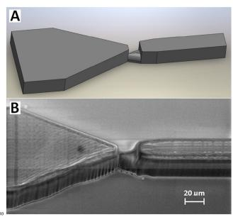
**Fig. 3** (A). CAD image of the 3-D structure that traps J2 *G. pallida.* (B) SEM image of the semi-cylindrical trapping channel. The rounded shape (written with the Nanoscribe) provides a tight fit to the contours of the worm.
