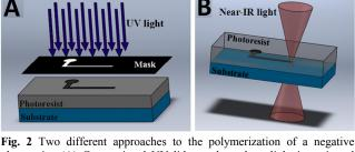
**Fig. 2** Two different approaches to the polymerization of a negative photoresist. (A) Conventional UV lithography, where light is projected <sup>90</sup> through a shadow mask onto a photosensitive material. (B) Two-photon polymerization: High resolution 3-D structures are written in the volume of the photoresist using a pulsed near-IR laser.
