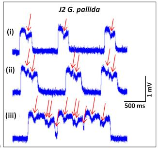
Fig. 7 Three different waveforms observed during recordings with StyletChip on J2 *G. pallida.* (i) Short thrust (ST): only two peaks generated during one single thrust with duration of ~ 300 ms. (ii) Normal thrust (NT): two to three peaks generated during one single thrust with <sup>20</sup> duration of ~500 ms. (iii) Rapid thrust (RT): several waveforms merged together to form one long thrust. Red arrows indicate the places of transient negative going potentials (TPs).
