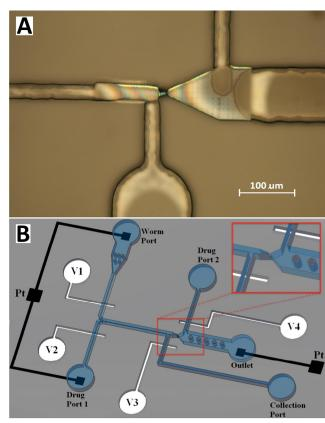
Fig. 4 (A) Photograph of the SU-8 master that is used to fabricate the <sup>65</sup> StyletChip. (B) Schematic layout of the chip showing the integrated Pt electrodes (at inlet and outlet), the trap region (inset) and the four valves (V1, V2, V3 and V4) used to control worm loading (V1), chemical or drug delivery (V2 and V4) and worm retrieval (V3).
