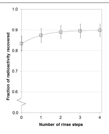
Figure 6. Effect of rinse steps on recovery of the concentrated radioactive sample from the chip. Here, a 10 mL sample of  $[^{18}F]FDG$  was concentrated. Data points show the average of three repetitions.
