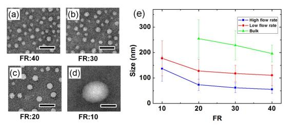
**Fig.3** TEM images of PLGA nanoparticles precipitated under different FRs. (a) middle channel: 10 mL/hr, each side channel: 200 mL/hr, and FR: 40, (b) middle channel: 13 mL/hr, each side channel: 198.5 mL/hr, and FR: 30, (c) middle channel: 20 mL/hr, each side channel: 195 mL/hr, and FR: 20, and (d) middle channel: 38 mL/hr, each side channel: 186 mL/hr, and FR: 10. The scale bar is 100 nm. (e) Size distribution of PLGA nanoparticles as a function s of FR by different approaches.
