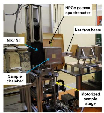
Fig. 2. The NIPS-NORMA station of the Budapest Neutron Centre
