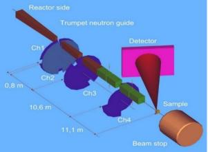
Fig. 3. The time-of-flight neutron diffractometer of the **Budapest Neutron Centre**
